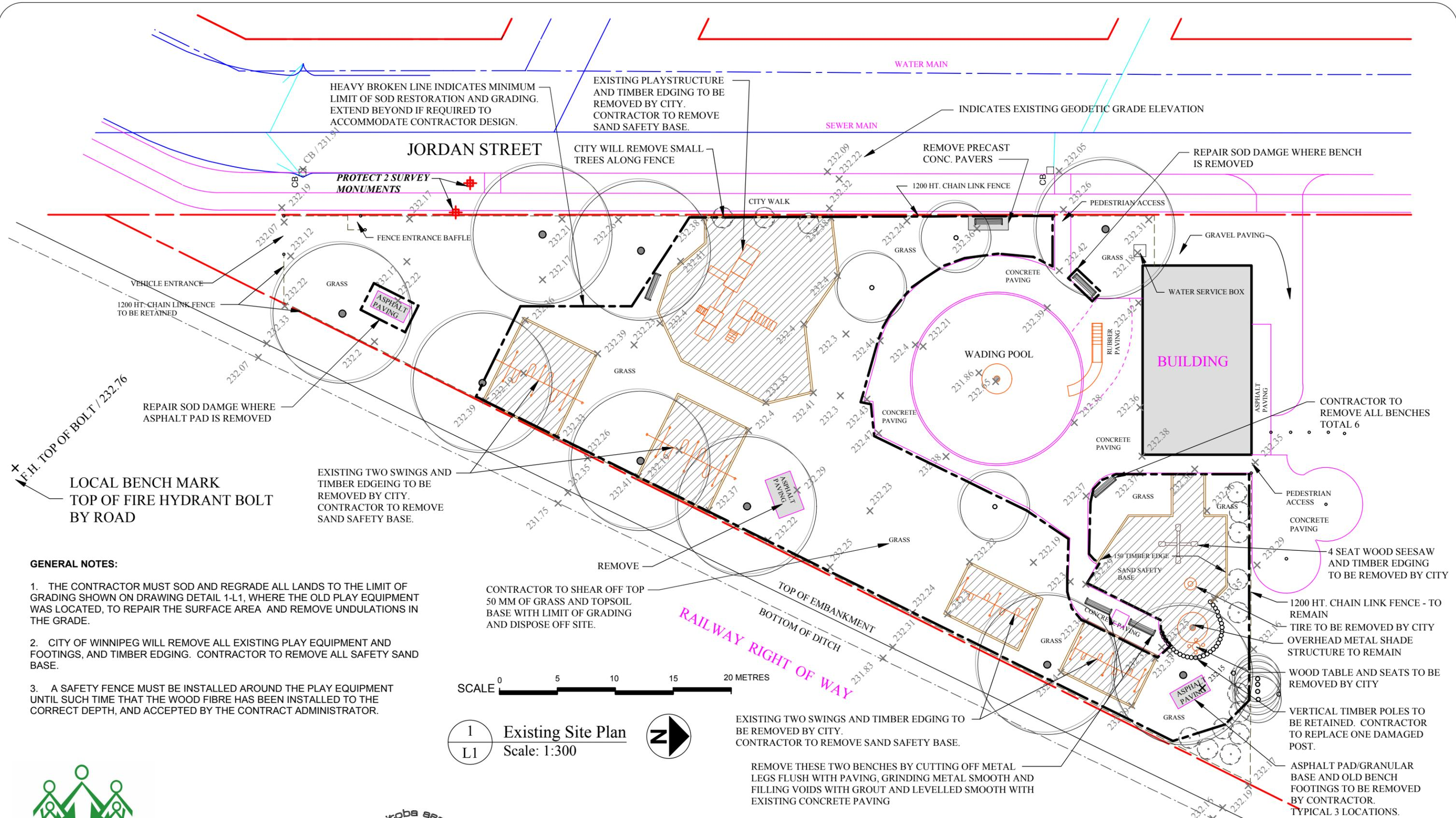
HEAVY BROKEN LINE INDICATES MINIMUM LIMIT OF SOD RESTORATION AND GRADING. EXTEND BEYOND IF REQUIRED TO ACCOMMODATE CONTRACTOR DESIGN.
