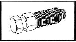
Adjustment is accomplished by rotating each of the three equally spaced adjusting sleeves counter clockwise by an equal amount, then tightening the clamping bolts onto them and checking for contact by rotating the shaft again. This step may have to be repeated a couple of times if the pump has some wear on it. Each flat of rotation of the adjustment sleeve hex nut is worth .010" to .012" of cutter movement. Typically the pump won't have more than .020" to .050" of wear.
