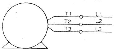
To reverse direction of rotation interchange any two line leads
