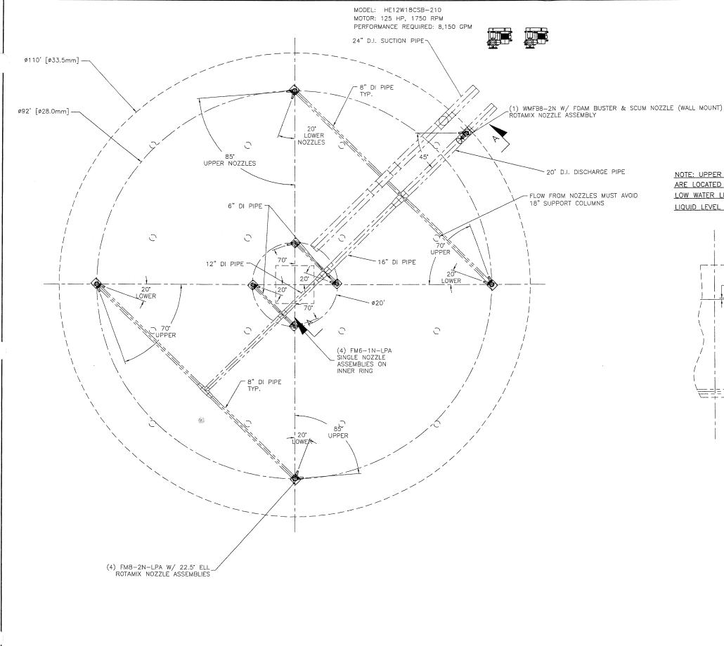
NOTE: UPPER SCUM NOZZLE MUST BE LOCATED SO THAT THEY ARE LOCATED 2 FEET BELOW LIQUID LEVEL AT LOW WATER LEVEL. NOZZLES MUST NOT DISCHARGE ABOVE LIQUID LEVEL TO AVOID POOR MIXING OR FOAMING.
