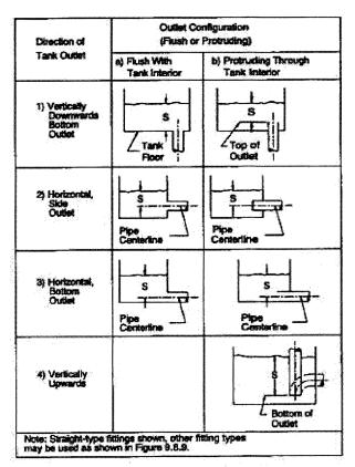
Figure 9.8.8 — Datum for calculation of submergence
