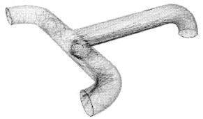
Fluid Dynamics (CFD) computer simulation study, showing swirling flow in both legs of a tee.
