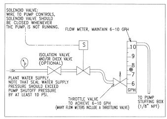
off with the pump motor. A schematic of this system is shown above.
