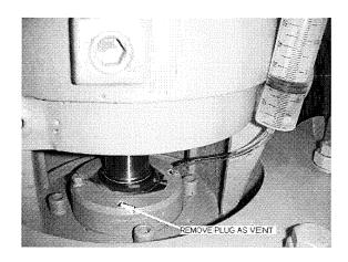
PE Pumps: Remove guard. Simply drain and refill using a syringe and tubing provided, with one plug removed as vent. Use 3 oz. of light oil (46 wt. hydraulic oil) to refill for 3"-6" pumps and 13 oz. for 8"-12" pumps. This will fill the seal approx. 3/4 full. Reinstall guard.
