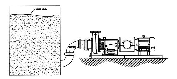
3) Avoid the use of tees near the pump on the suction side piping. Tees induce swirling flow in the piping downstream of the tee, causing reweaving of hair and fiber into rags, which can then plug pumps. Plugging on re-woven rags is less of a problem with chopper pumps, but the swirling flow also hurts pump performance. Y-type fittings provide considerably better flow. Below is an image of a Computational
