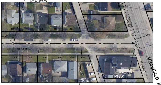
103.80 OF 300 CONC CS TO BE LINED S-MA50007732 (FULLY DETERIORATED)
