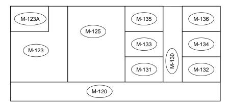
Figure 3-1: Room Numbering on Drawings - Plan View
