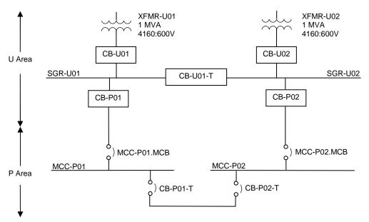
Figure 6-1 : Sample Tie Breaker Identification
