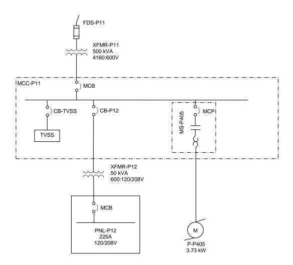
Figure 6-2 : Subcomponents – Electrical Equipment
