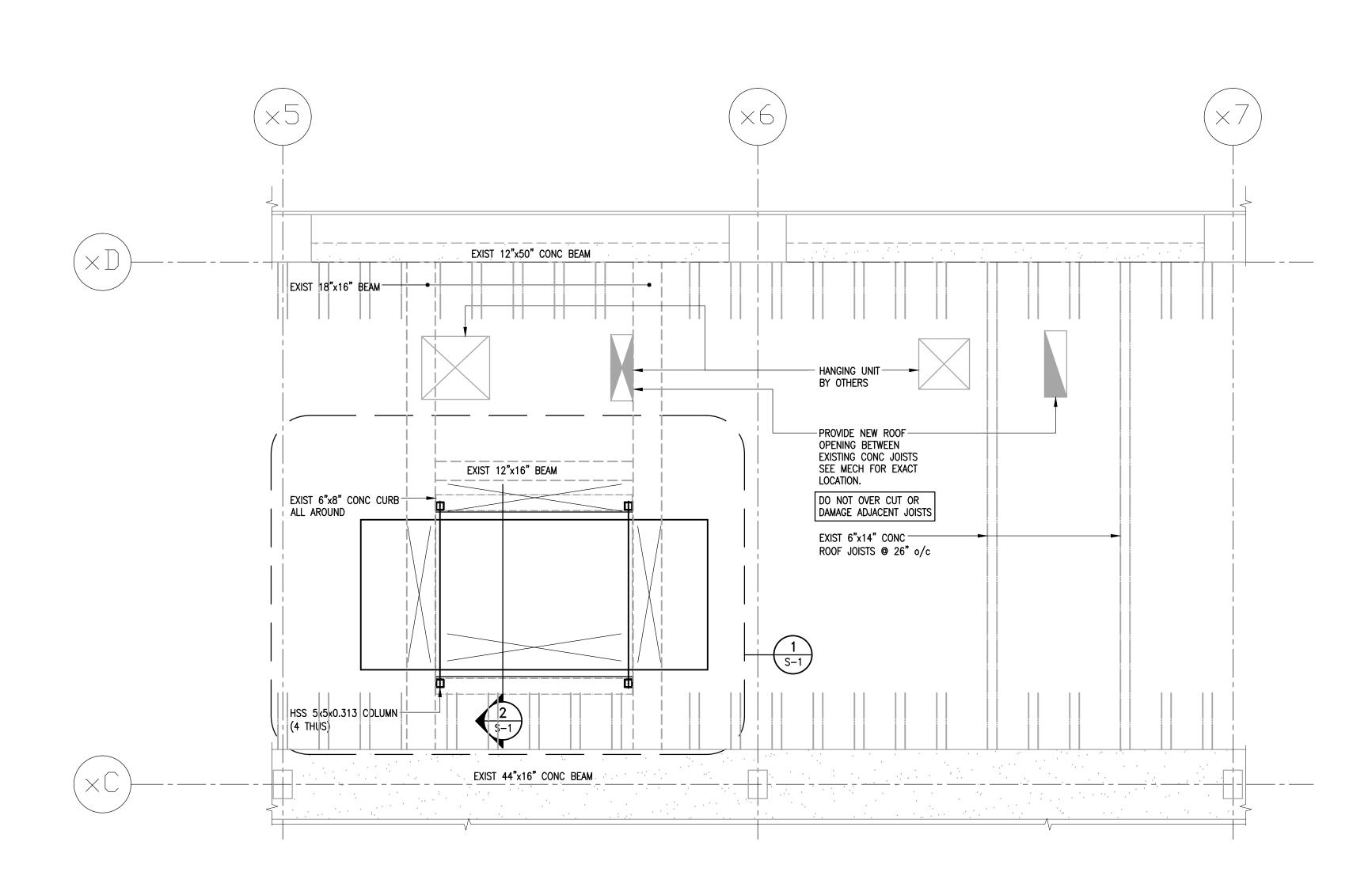
PARTIAL ROOF PLAN - NEW CONSTRUCTION • REMOVAL OF EXISTING COOLING TOWER UNIT AND FRAMING BY OTHERS. DO NOT DAMAGE EXISTING CONCRETE FRAMING AROUND OPENING. DESIGN ROOF LIVE LOAD = 36 PSF
