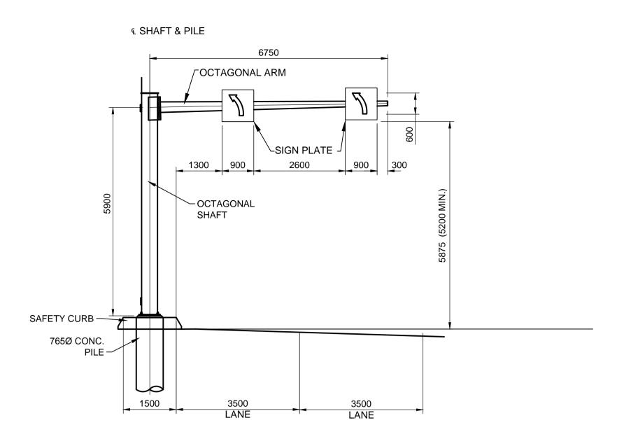
ELEVATION - LOOKING EAST OVERHEAD SIGN SUPPORT STRUCTURE NO. S768
