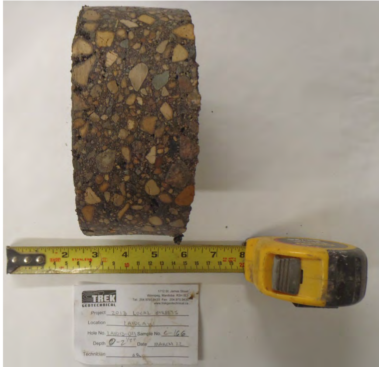
Photo 7: Asphalt Core Sample from Test Hole LAID13-04
