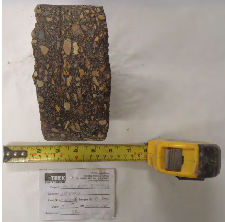
Photo 15: Asphalt Core Sample from Test Hole LAID13-08
