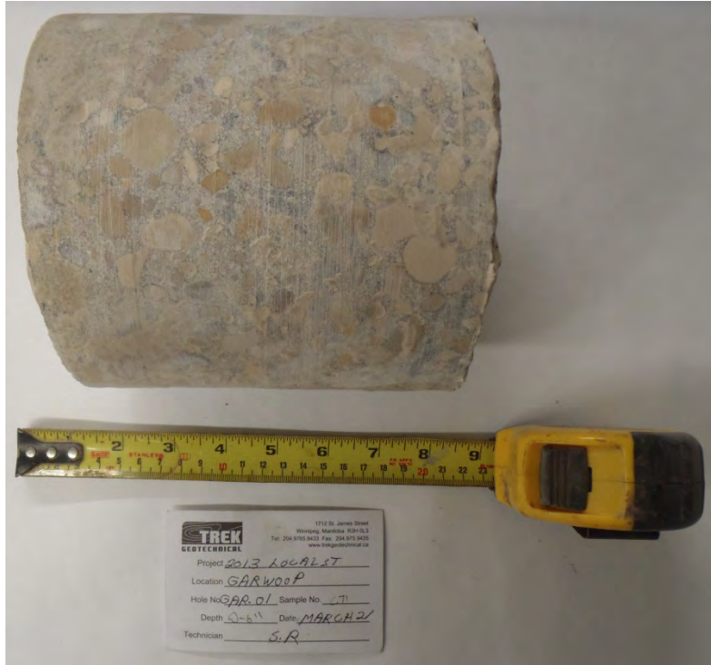
Photo 1: Concrete Core Sample from Test Hole GAR13-01
