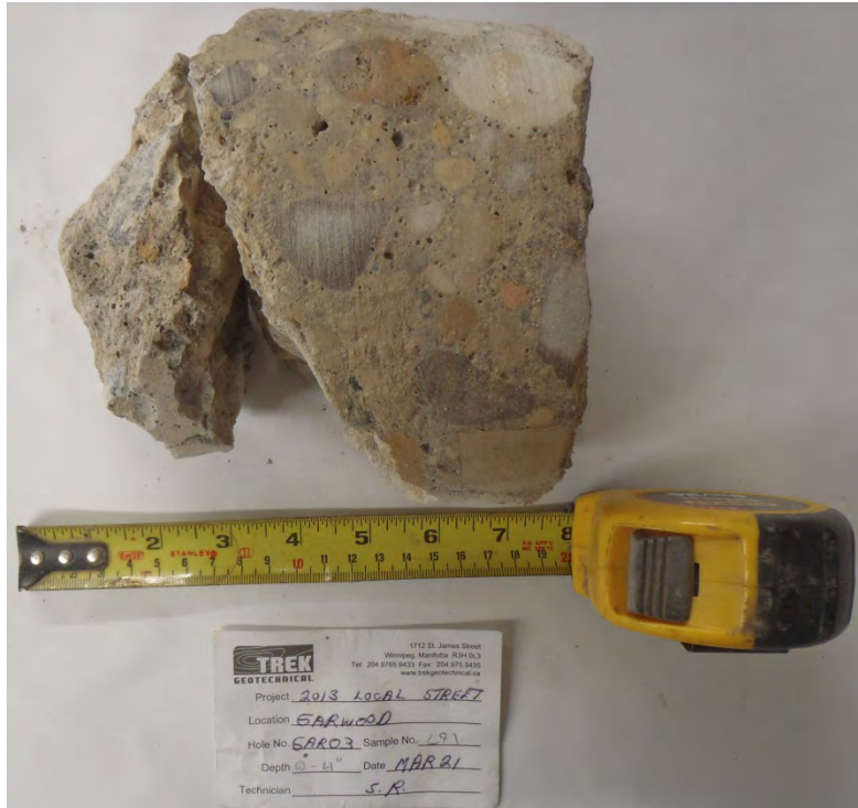
Photo 3: Concrete Core Sample from Test Hole GAR13-03
