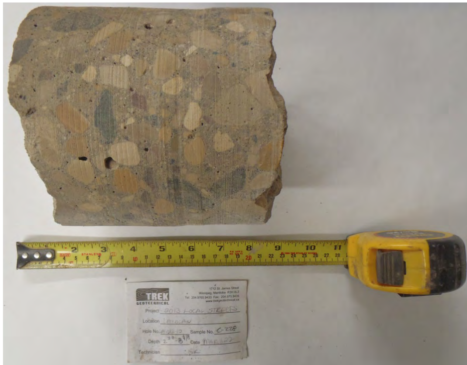
Photo 20: Concrete Core Sample from Test Hole LAID13-10
