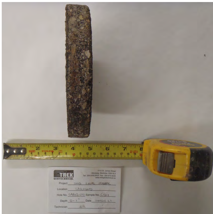
Photo 4: Asphalt Core Sample from Test Hole GAR13-04
