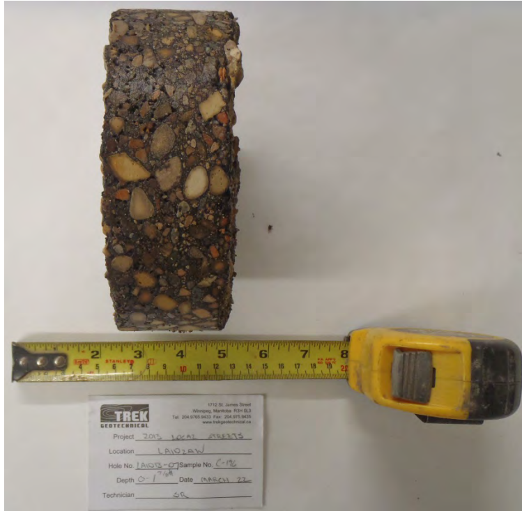
Photo 13: Asphalt Core Sample from Test Hole LAID13-07
