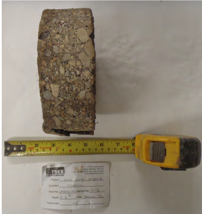
Photo 9: Asphalt Core Sample from Test Hole LAID13-05
