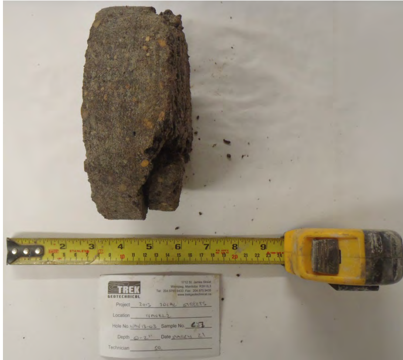
Photo 3: Asphalt Core sample from Test Hole WAV13-03
