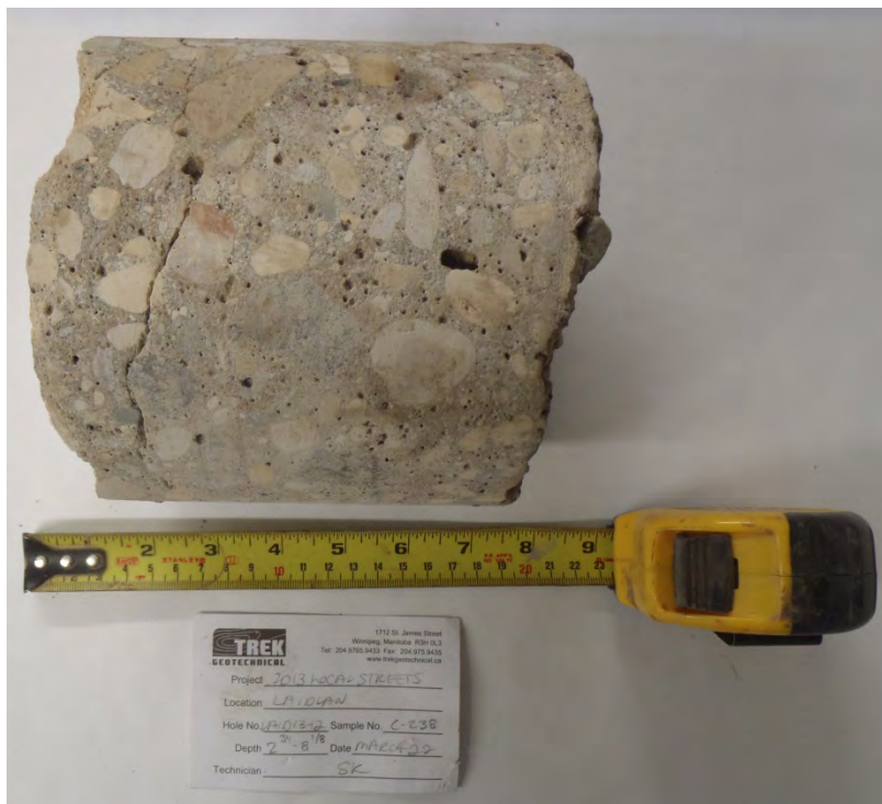
Photo 24: Concrete Core Sample from Test Hole LAID13-12
