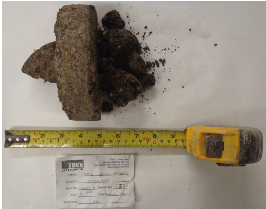
Photo 21: Asphalt Core Sample from Test Hole LAID13-11
