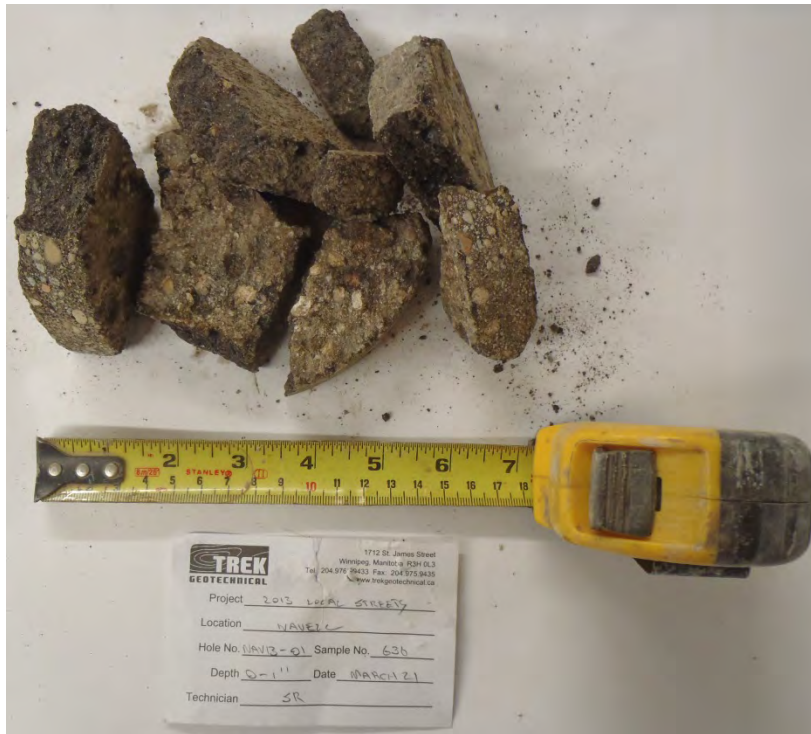
Photo 1: Asphalt Core Sample from Test Hole WAV13-01
