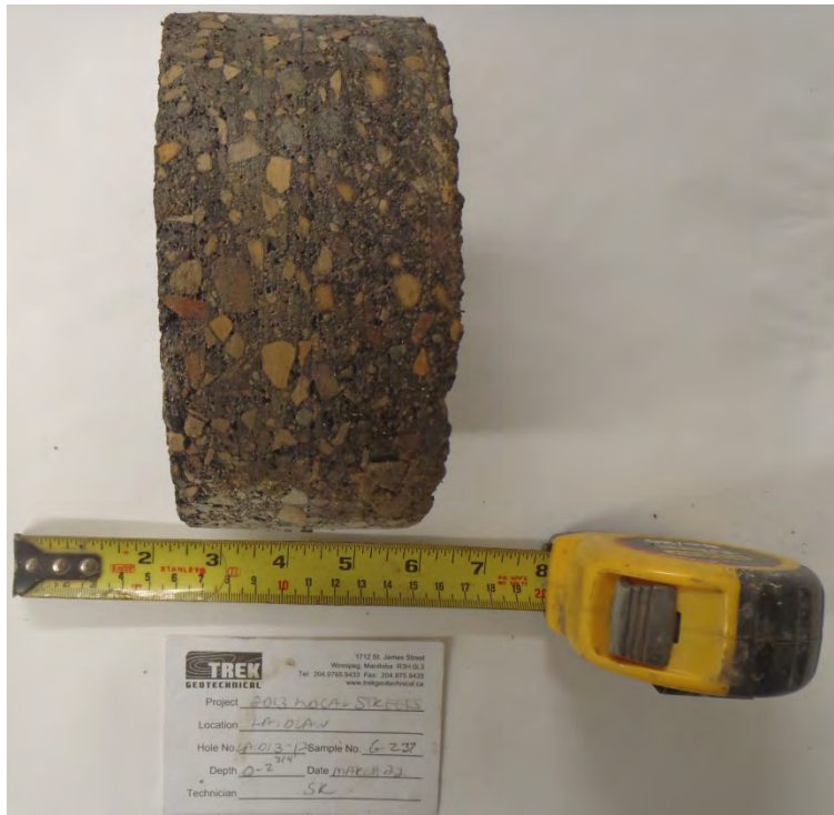
Photo 23: Asphalt Core Sample from Test Hole LAID13-12
