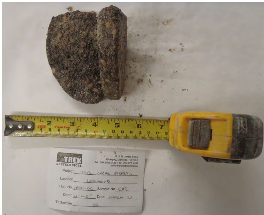
Photo 6: Asphalt Core Sample from Test Hole GAR13-05
