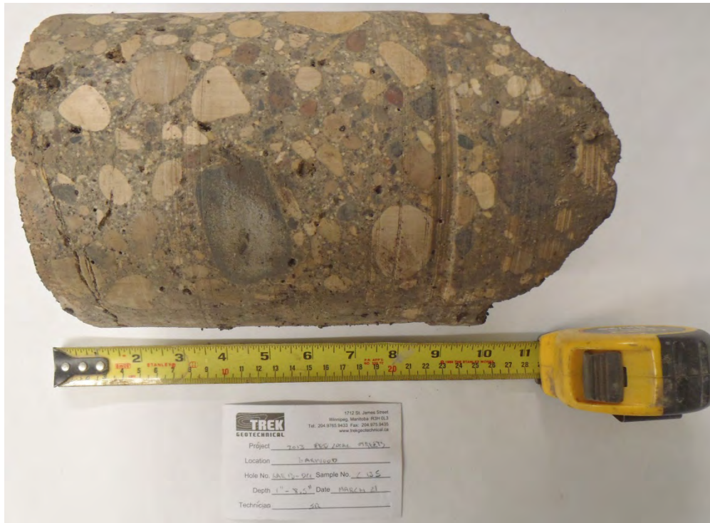
Photo 5: Concrete Core Sample from Test Hole GAR13-04
