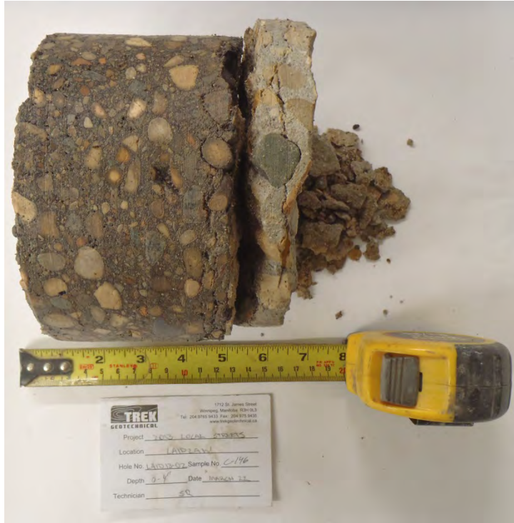
Photo 3: Asphalt and Concrete Core Sample from Test Hole LAID13-02
