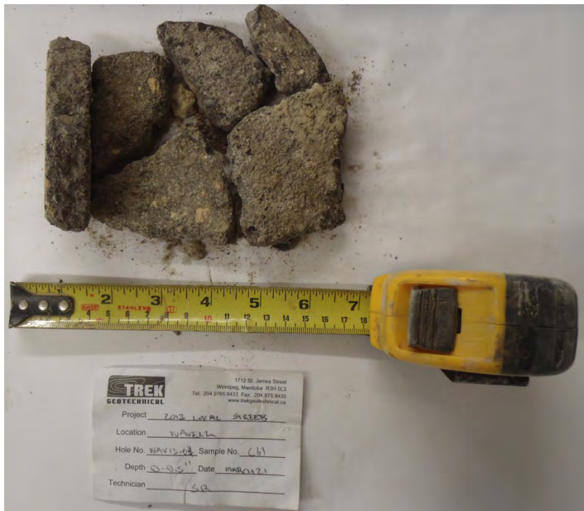
Photo 4: Asphalt Core sample from Test Hole WAV13-04
