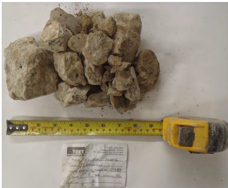
Photo 22: Concrete Core Sample from Test Hole LAID13-11
