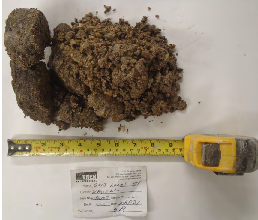
Photo 7: Asphalt and Concrete core sample from Test Hole WAV13-07
