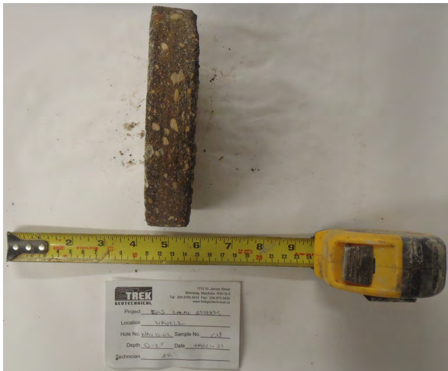
Photo 2: Asphalt Core Sample from Test Hole WAV13-02
