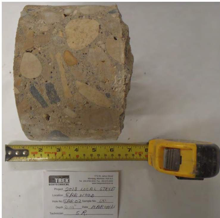
Photo 2: Concrete Core Sample from Test Hole GAR13-02
