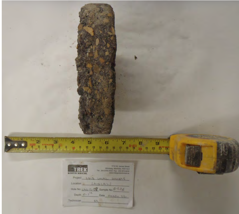
Photo 17: Asphalt Core Sample from Test Hole LAID13-09
