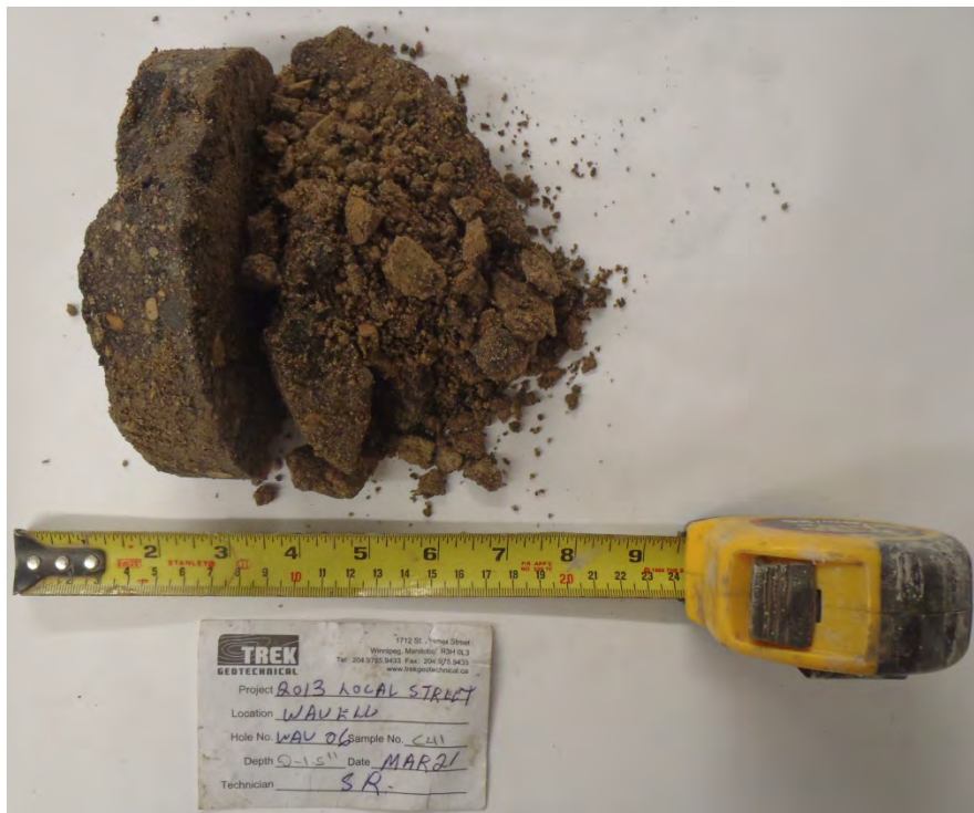
Photo 6: Asphalt Core sample from Test Hole WAV13-06
