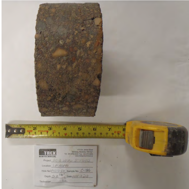
Photo 11: Asphalt Core Sample from Test Hole LAID13-06
