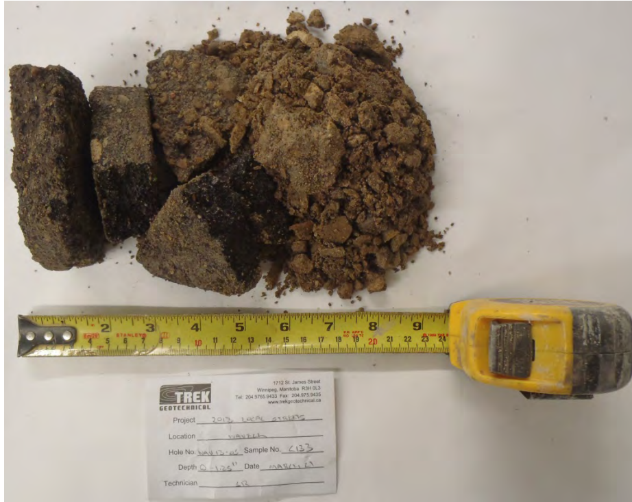
Photo 5: Asphalt and Concrete Core sample from Test Hole WAV13-05
