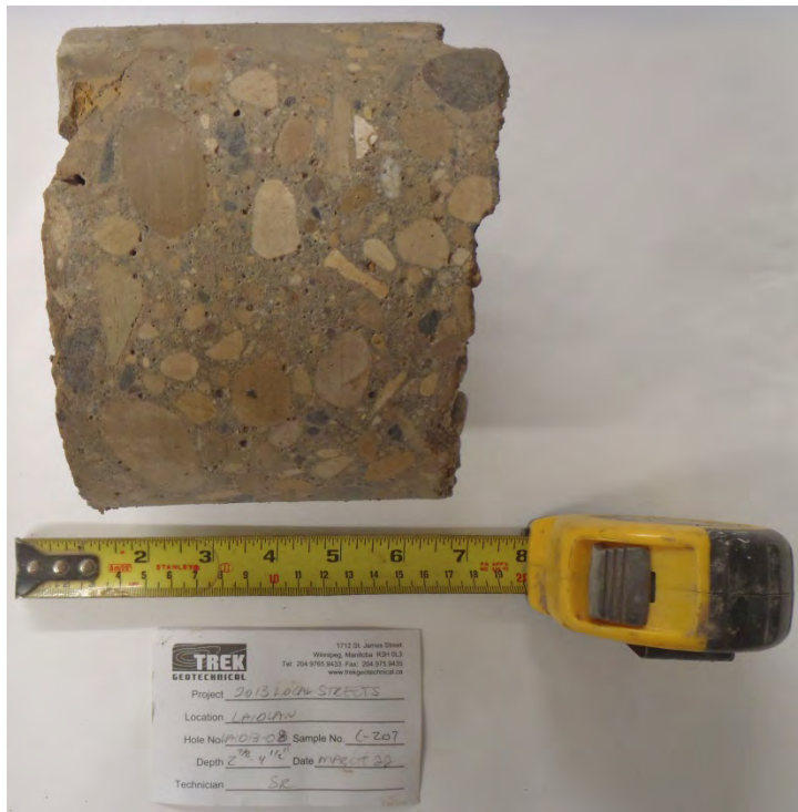
Photo 16: Concrete Core Sample from Test Hole LAID13-08
