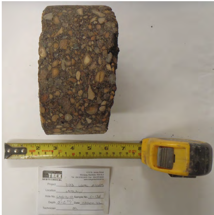
Photo 1: Asphalt Core Sample from Test Hole LAID13-01
