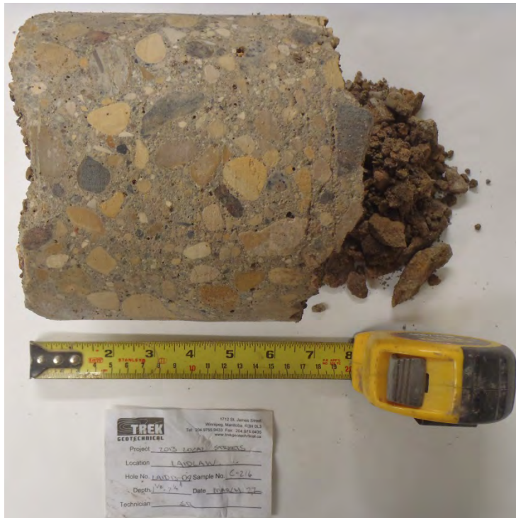
Photo 18: Concrete Core Sample from Test Hole LAID13-09
