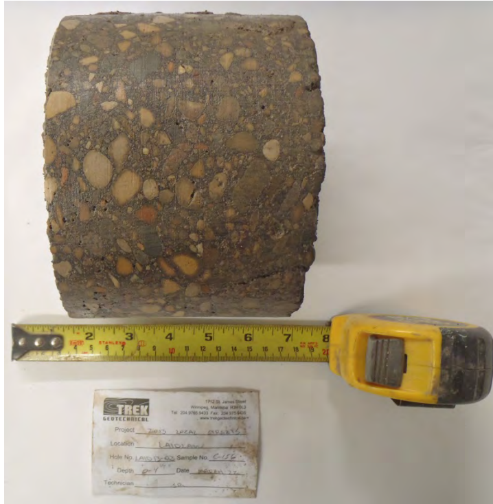
Photo 5: Asphalt Core Sample from Test Hole LAID13-03
