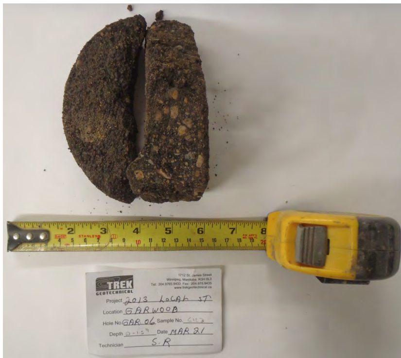
Photo 8: Asphalt Core Sample from Test Hole GAR13-06
