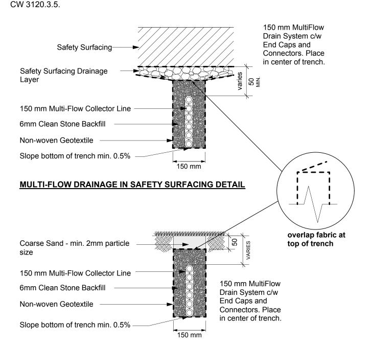
**MULTI-FLOW DRAINAGE IN TURF DETAIL**
