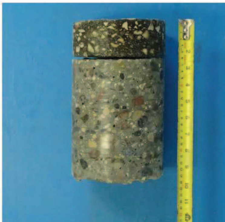
Core sample from Testhole TH4
