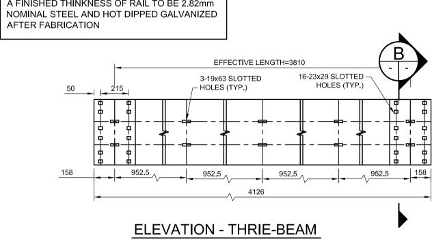
A FINISHED THINKNESS OF RAIL TO BE 2.82mm NOMINAL STEEL AND HOT DIPPED GALVANIZED AFTER FABRICATION
