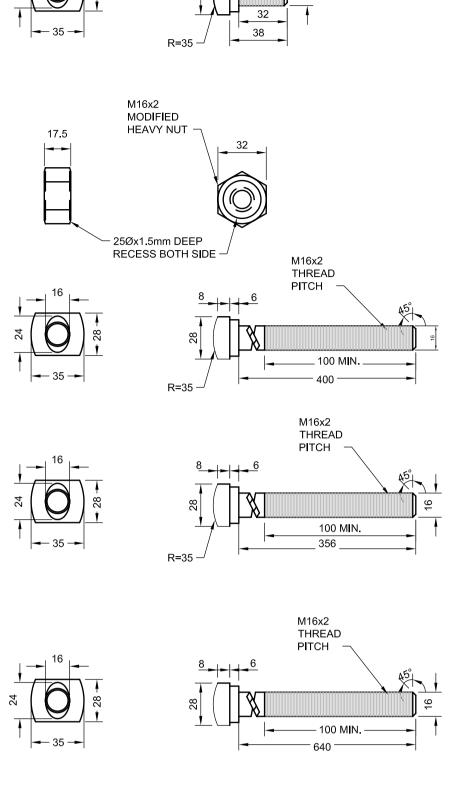
GUARDRAIL BOLT AND RECESSED NUT
