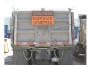
Amber Strobe light at top, with brake/signal/backup light array in side configuration
