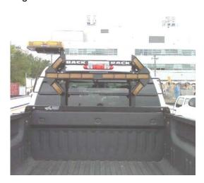
Directional Arrows and beacon/strobe for increased visibility, used as a blocking/shadowing vehicle
