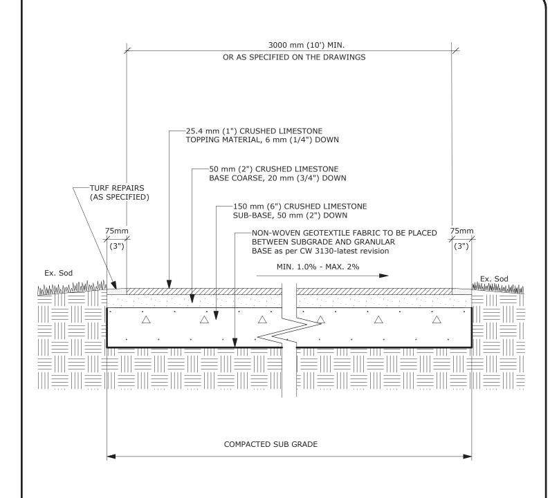
DIMENSIONS SHOWN ARE IN MILLIMETRES UNLESS OTHERWISE SPECIFIED
