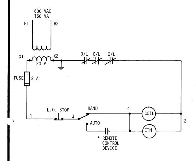
\* REMOTE CONTROL DEVICE IS P.B. RELAY IN SOLID STATE ALTERNATOR
