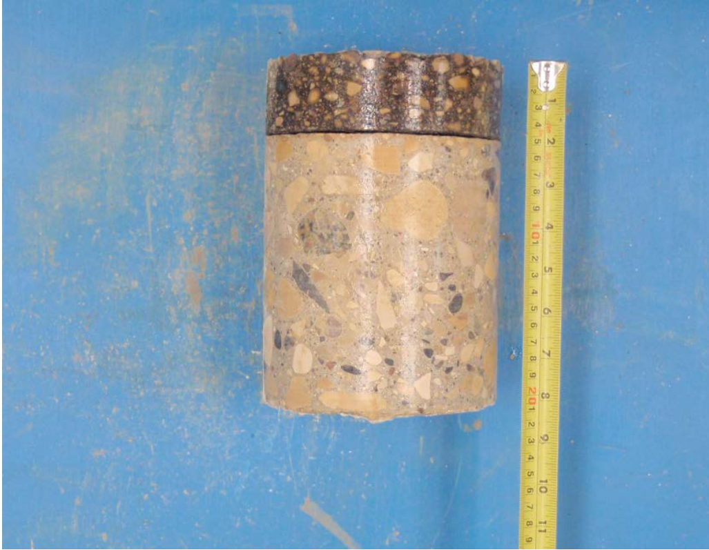
Core sample from Testhole TH05
