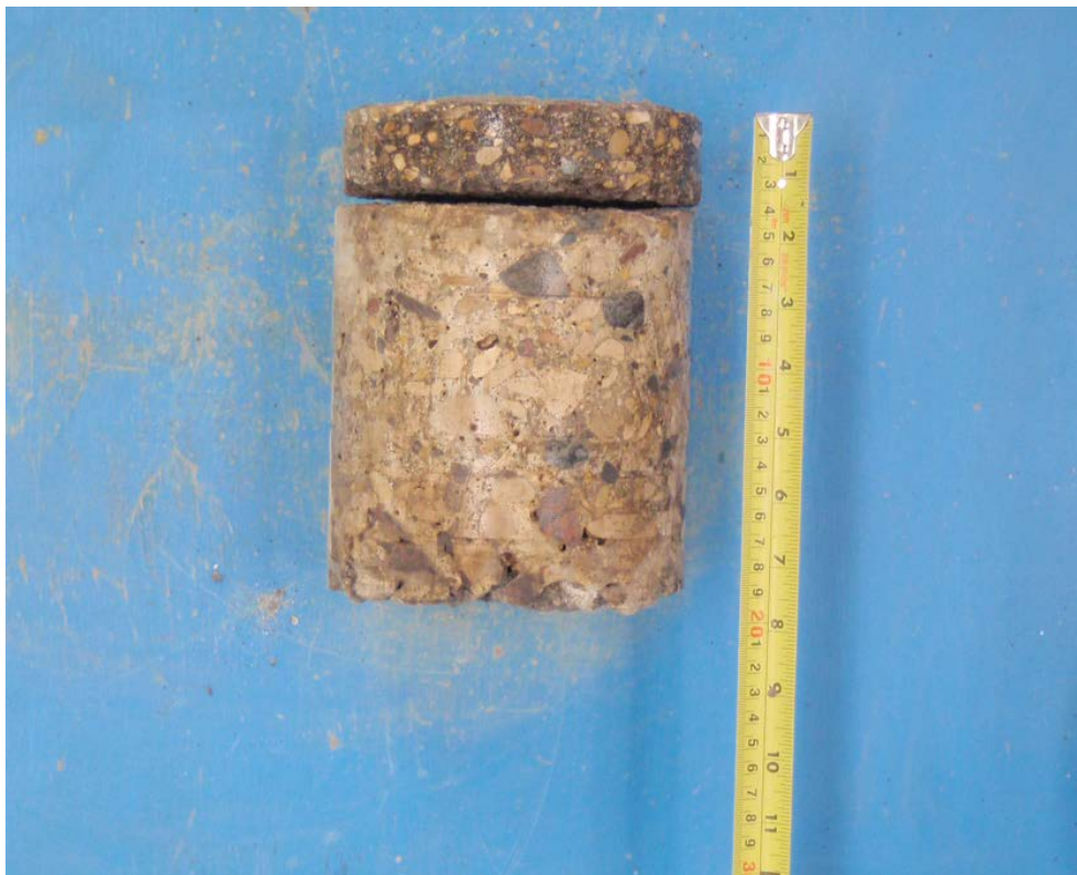
Core sample from Testhole TH10
