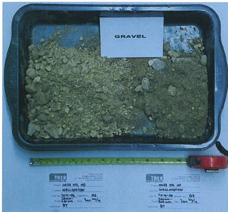
Photo 14: 19 mm Down Limestone over Sand and Gravel (A-Base) Sample from Test Hole TH14-06
