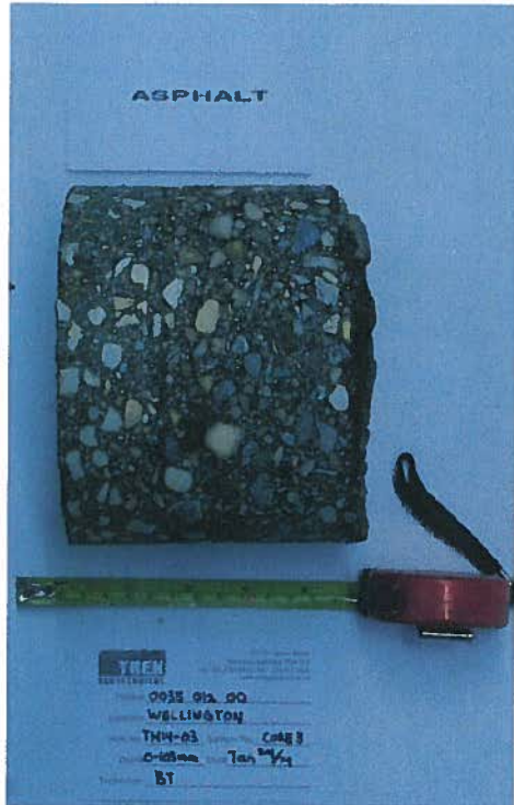
Photo 5: Asphalt Core Sample from Test Hole TH14-03
