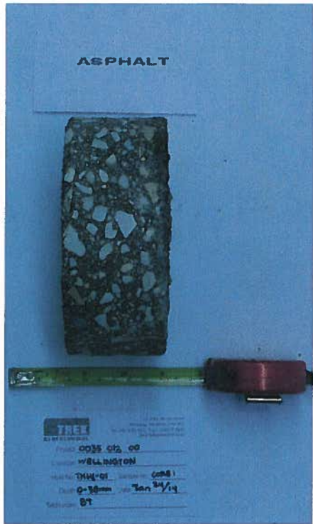
Photo 1: Asphalt Core Sample from Test Hole TH14-01
