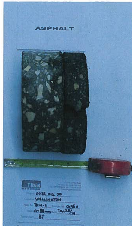
Photo 23: Asphalt Core Sample from Test Hole TH14-11
