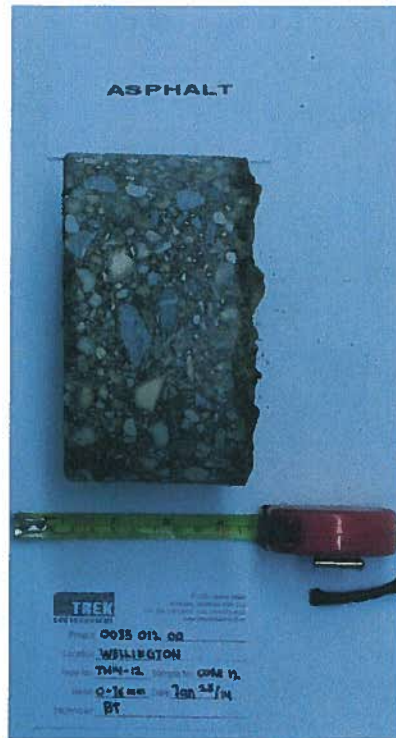
Photo 25: Asphalt Core Sample from Test Hole TH14-12
