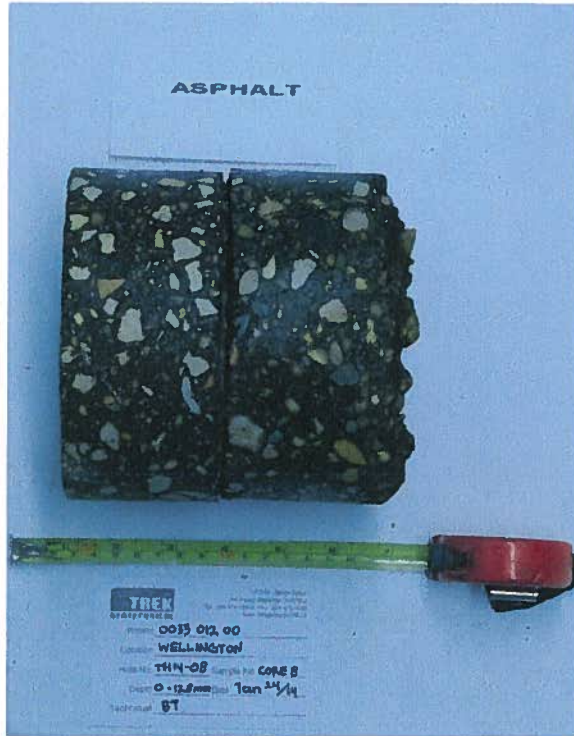
Photo 17: Asphalt Core Sample from Test Hole TH14-08
