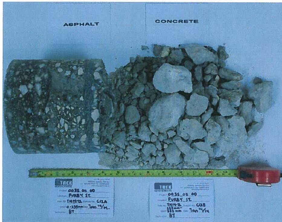
Photo 4: Asphalt and Concrete Core Sample from Test Hole TH14-12
