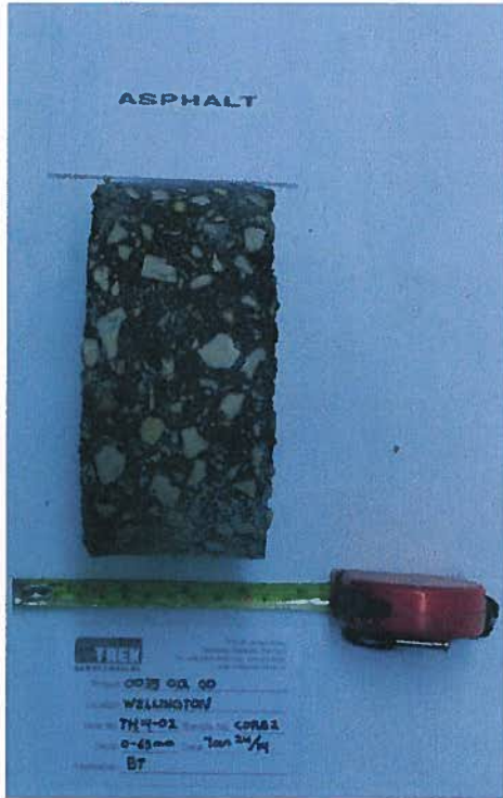
Photo 3: Asphalt Core Sample from Test Hole TH14-02
