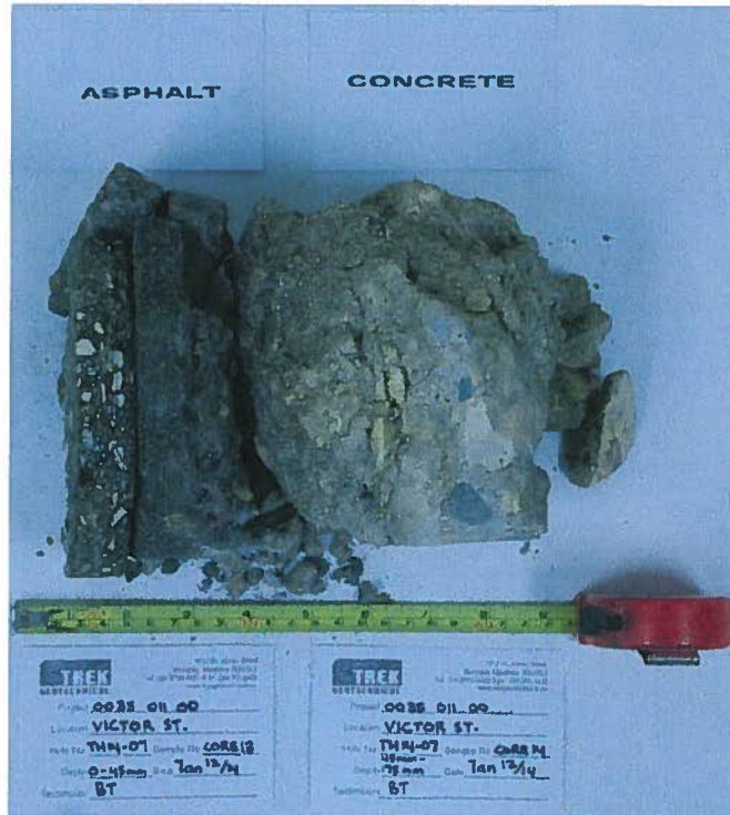
Photo 7: Asphalt and Concrete Core Sample from Test Hole TH14-07
