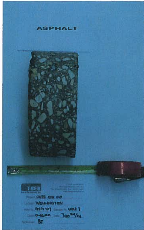
Photo 15: Asphalt Core Sample from Test Hole TH14-07
