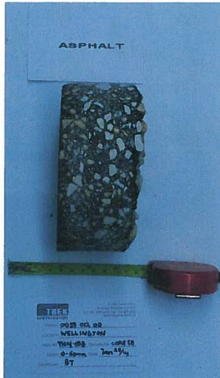
Photo 11: Asphalt Core Sample from Test Hole TH14-05B
