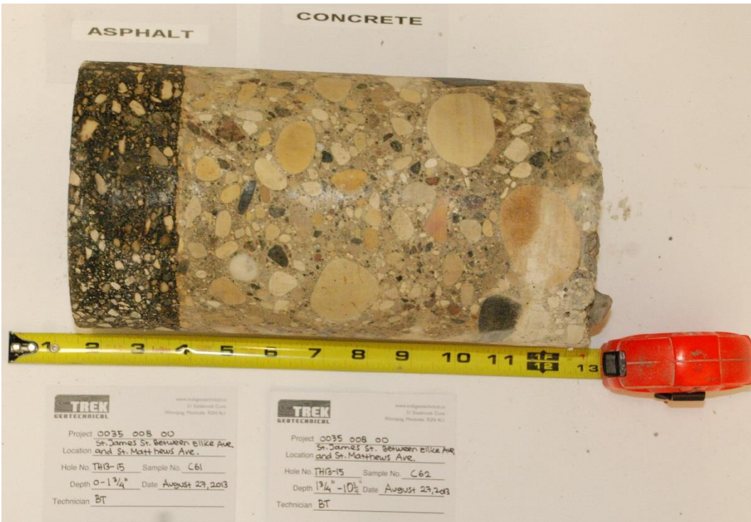
Photo 12: Asphalt and Concrete Core Sample from Test Hole TH13-15
