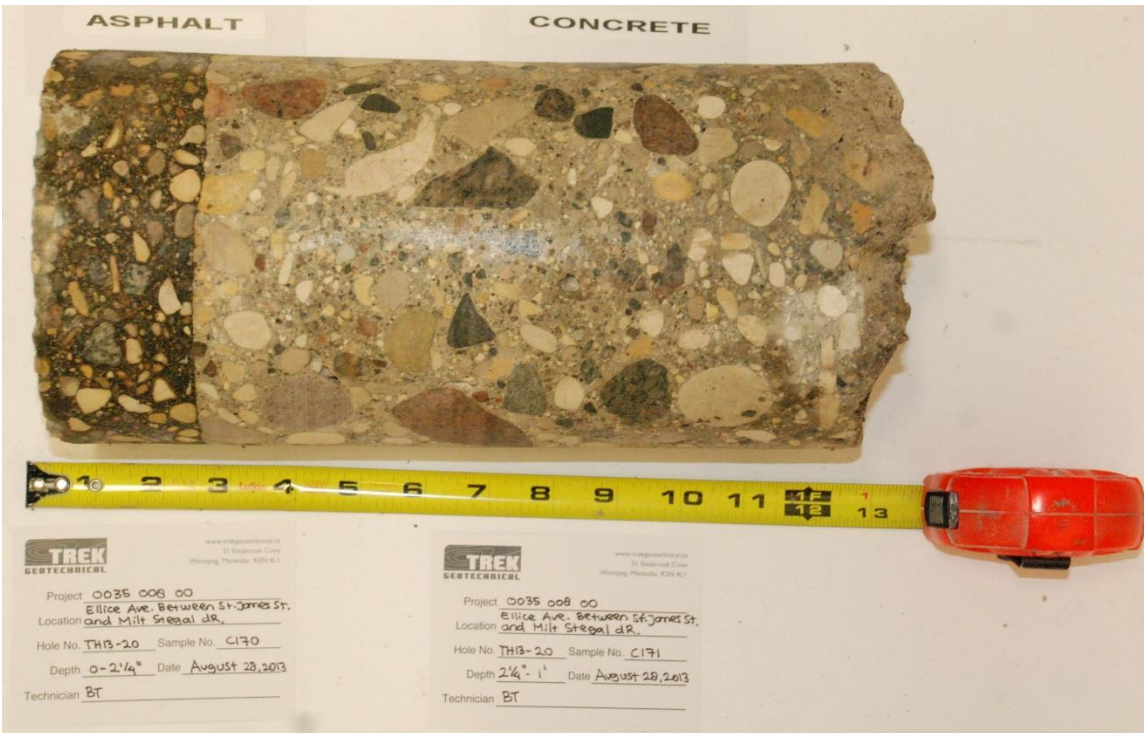
Photo 18: Asphalt and Concrete Core Sample from Test Hole TH13-20
