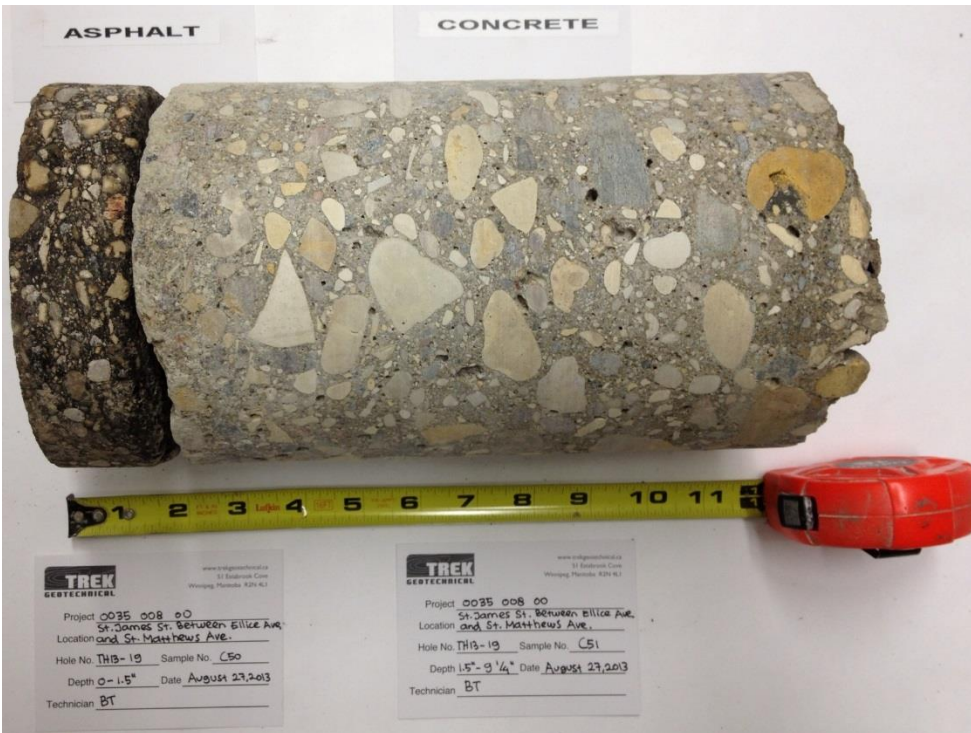
Photo 16: Asphalt and Concrete Core Sample from Test Hole TH13-19
