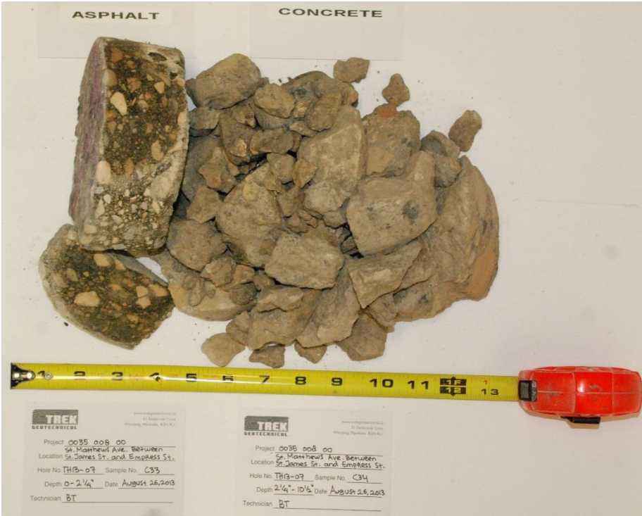
Photo 5: Asphalt and Concrete Core Sample from Test Hole TH13-07
