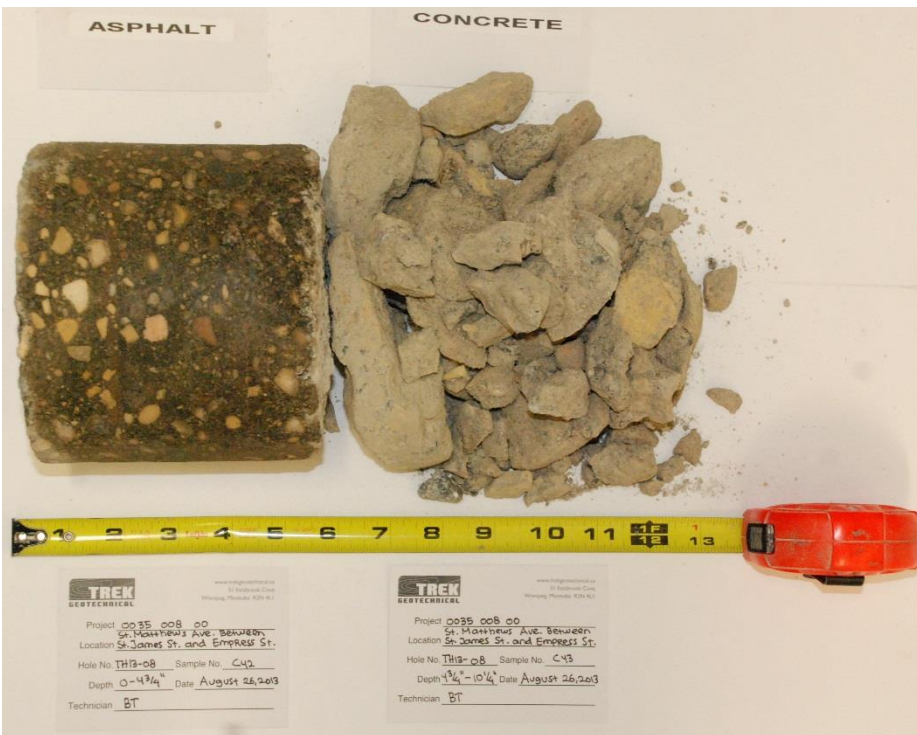
Photo 6: Asphalt and Concrete Core Sample from Test Hole TH13-08
