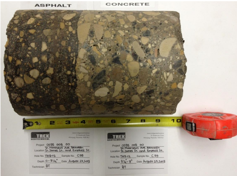
Photo 9: Asphalt and Concrete Core Sample from Test Hole TH13-12
