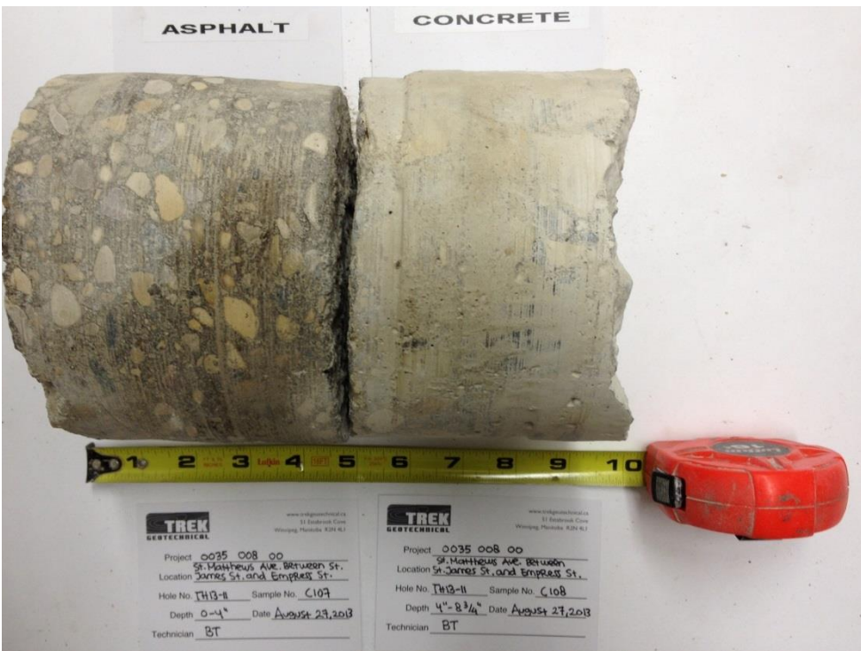
Photo 8: Asphalt and Concrete Core Sample from Test Hole TH13-11
