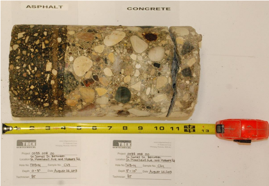
Photo 11: Asphalt and Concrete Core Sample from Test Hole TH13-14
