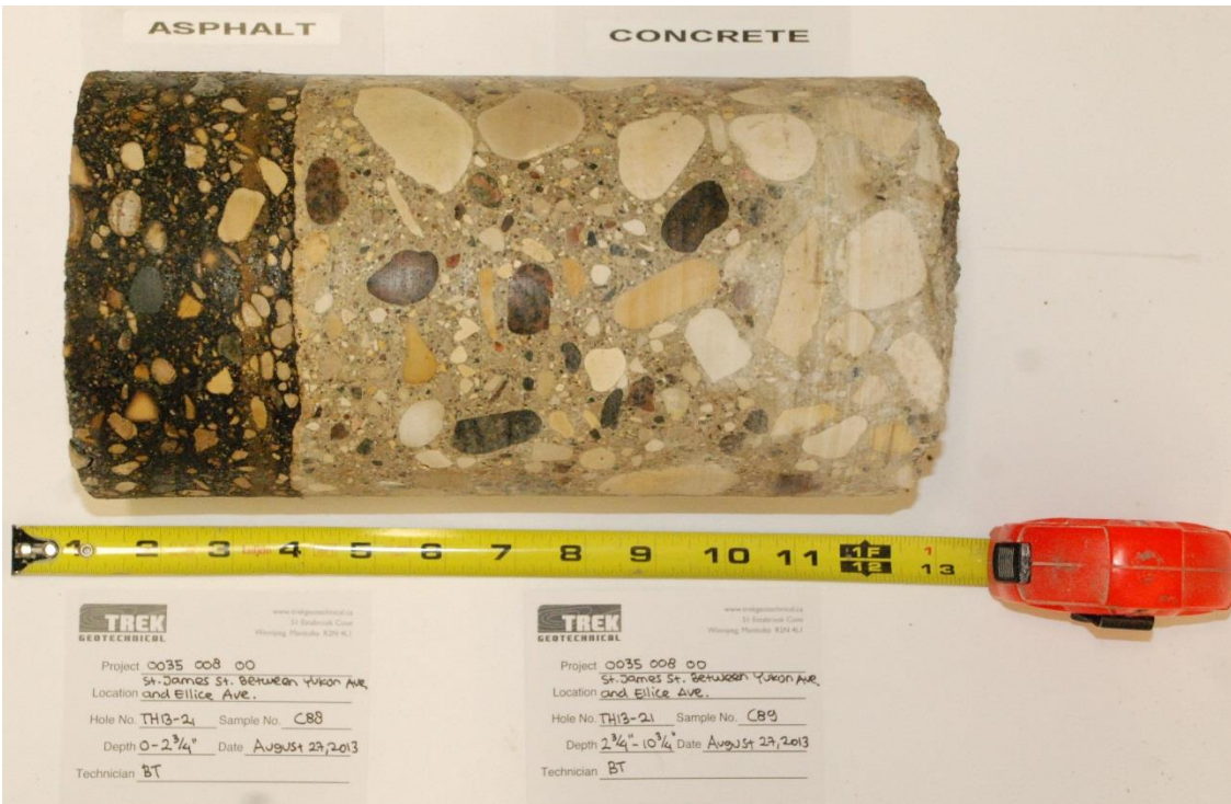
Photo 19: Asphalt and Concrete Core Sample from Test Hole TH13-21
