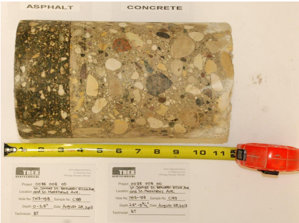
Photo 17: Asphalt and Concrete Core Sample from Test Hole TH13-19B
