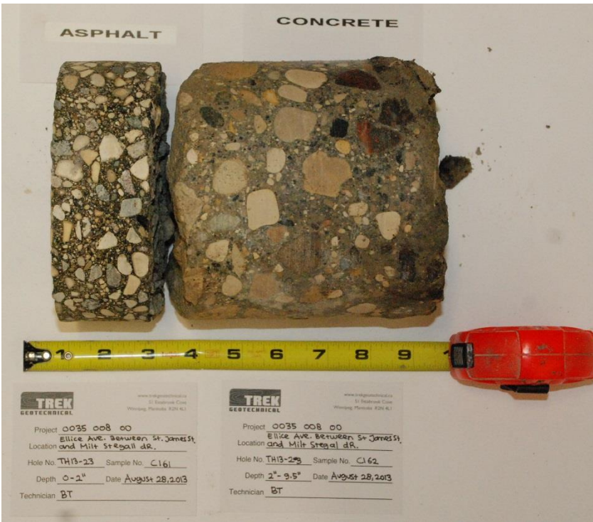
Photo 21: Asphalt and Concrete Core Sample from Test Hole TH13-23
