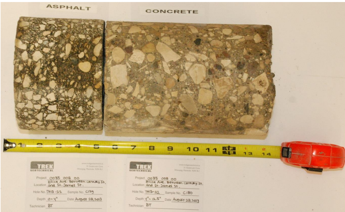
Photo 20: Asphalt and Concrete Core Sample from Test Hole TH13-22
