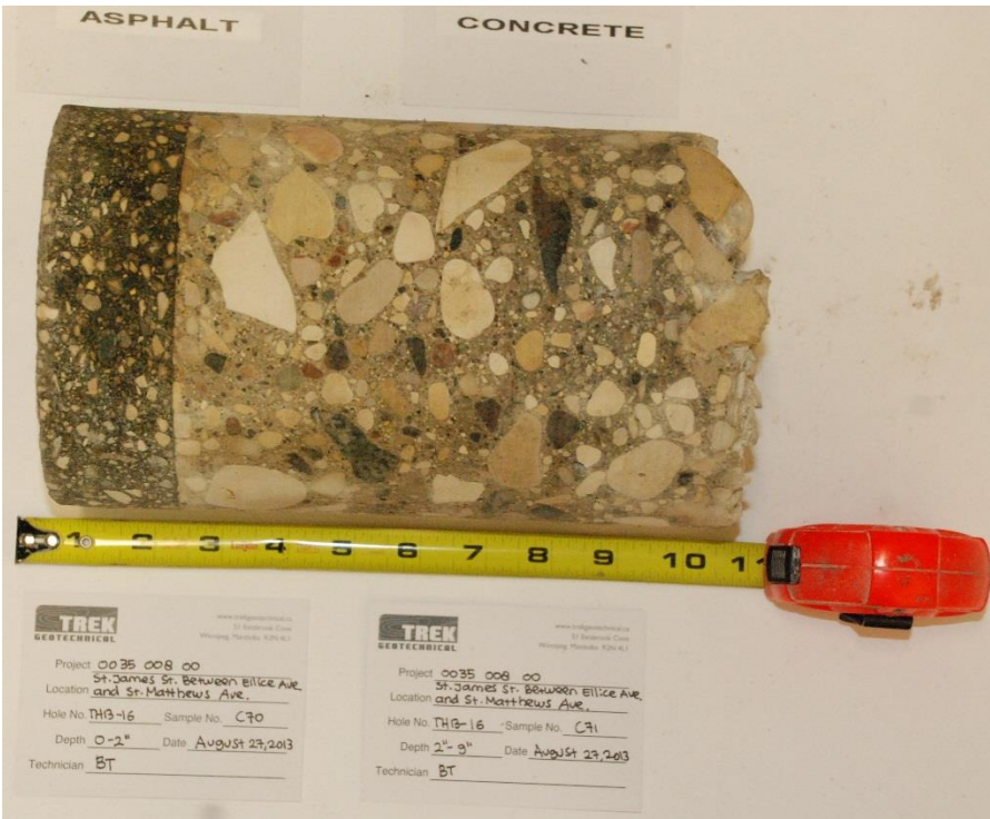
Photo 13: Asphalt and Concrete Core Sample from Test Hole TH13-16
