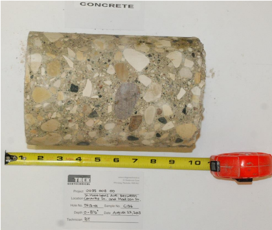
Photo 1: Concrete Core Sample from Test Hole TH13-01
