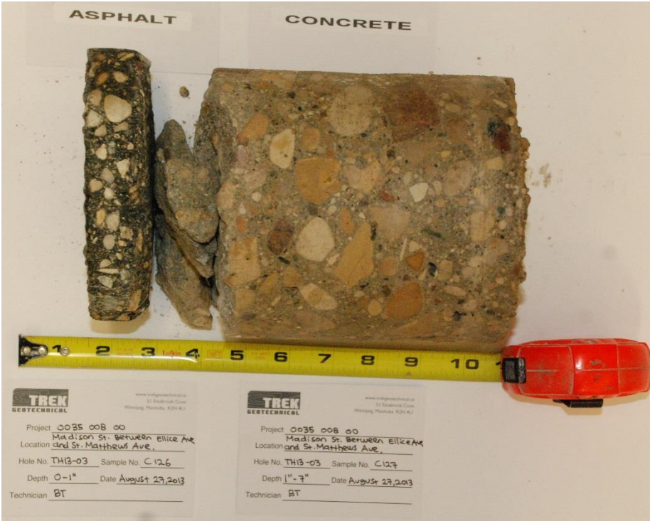
Photo 3: Asphalt and Concrete Core Sample from Test Hole TH13-03
