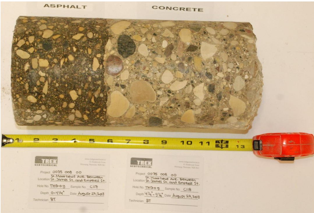
Photo 7: Asphalt and Concrete Core Sample from Test Hole TH13-09
