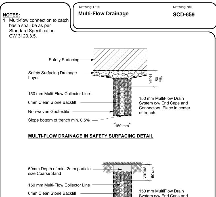
150 mm MultiFlow Drain System c/w End Caps and Connectors. Place in center of trench.
