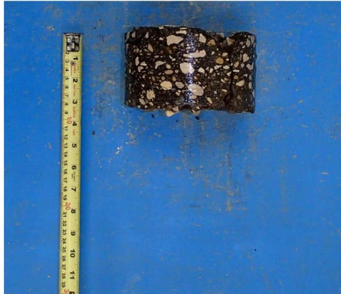
Core sample from Testhole TH4
