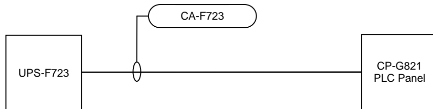
Figure 7-2: Instrument Cable Identification Example – Identified Equipment
