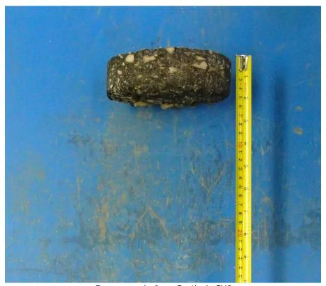
Core sample from Testhole TH2
