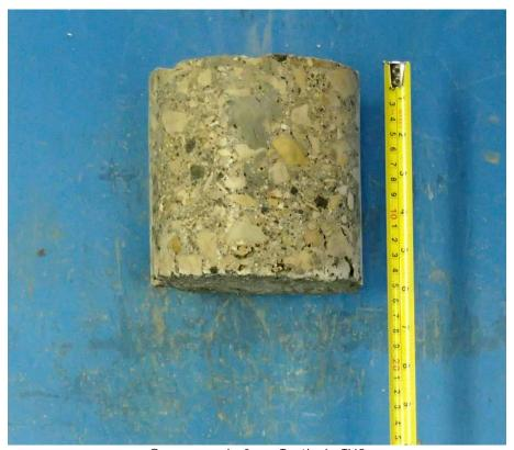
Core sample from Testhole TH2
