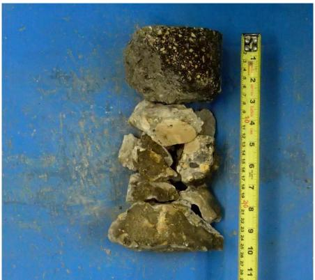
Core sample from Testhole TH2
