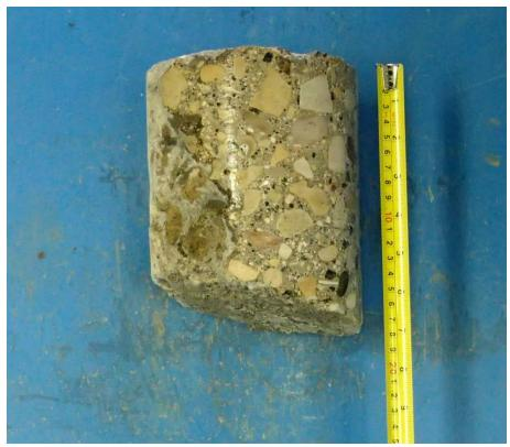
Core sample from Testhole TH3
