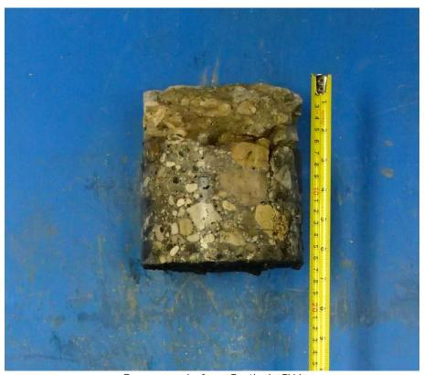
Core sample from Testhole TH4
