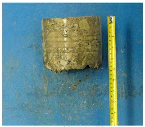
Core sample from Testhole TH4
