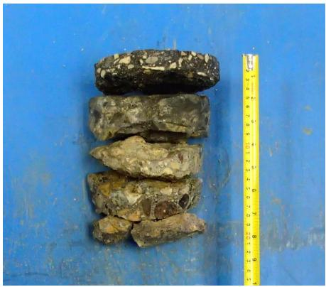
Core sample from Testhole TH3
