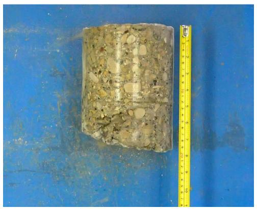
Core sample from Testhole TH8
