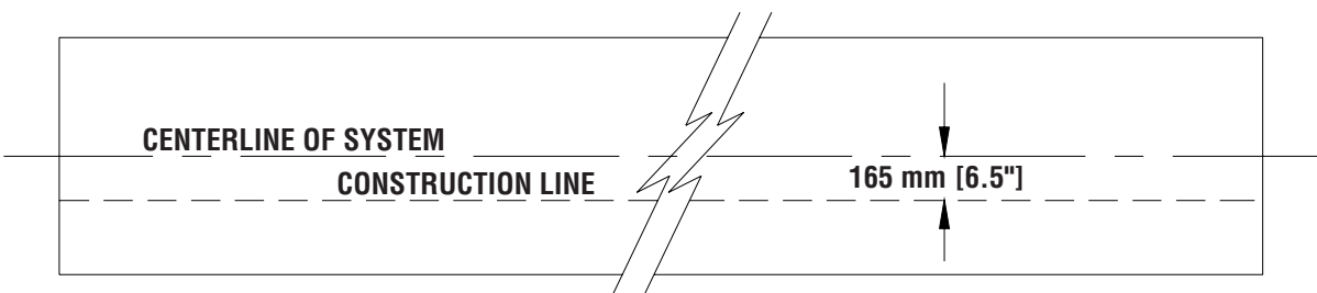
Figure 46 (Top view of Concrete Pad) Locating Construction Line
