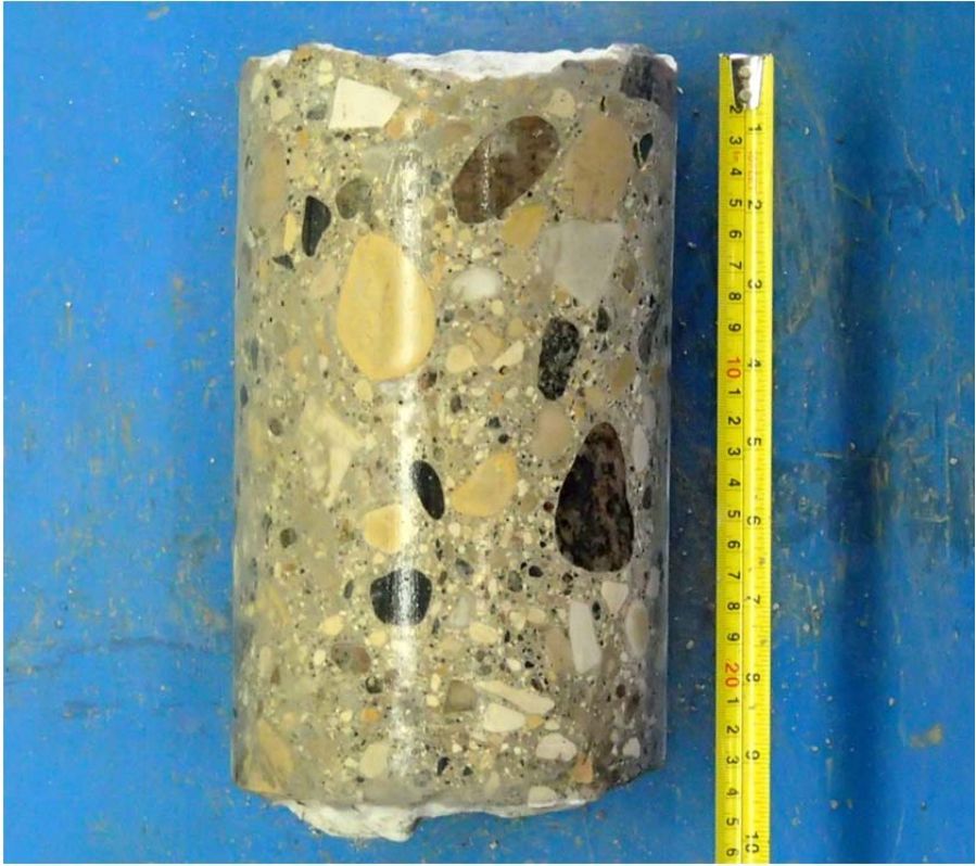
Core sample from Testhole TH3
