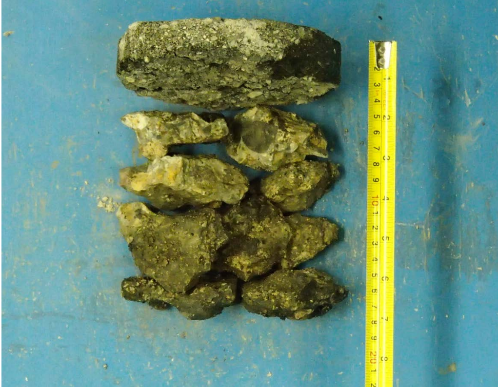
Core sample from Testhole TH5
