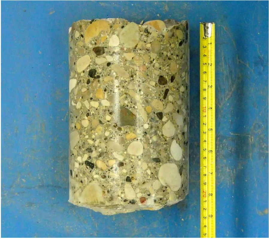
Core sample from Testhole TH6
