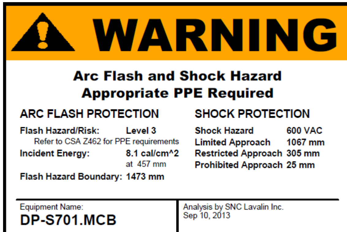
Figure 12-2 : Arc Flash Warning Label, Category 0 through 4 - Large
