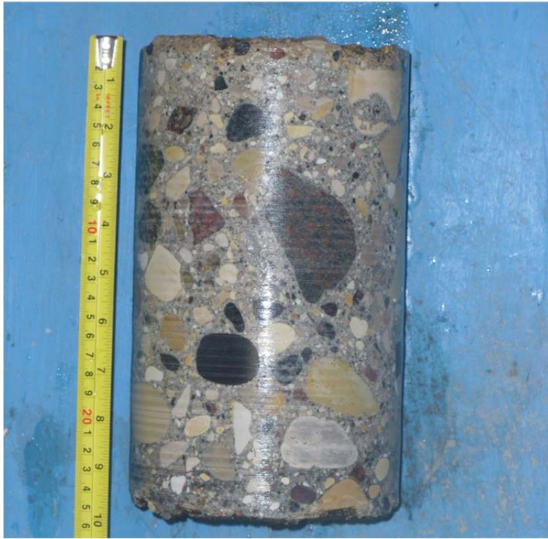
Core sample from Testhole TH3
