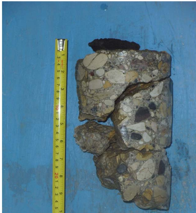
Core sample from Testhole TH4
