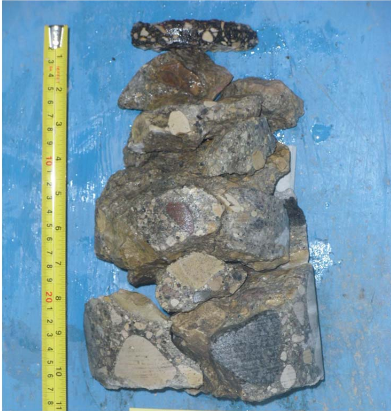
Core sample from Testhole TH1
