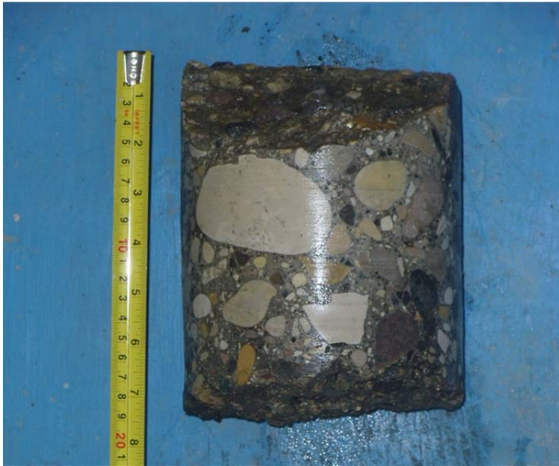
Core sample from Testhole TH3
