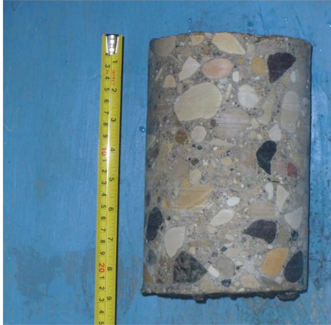
Core sample from Testhole TH1
