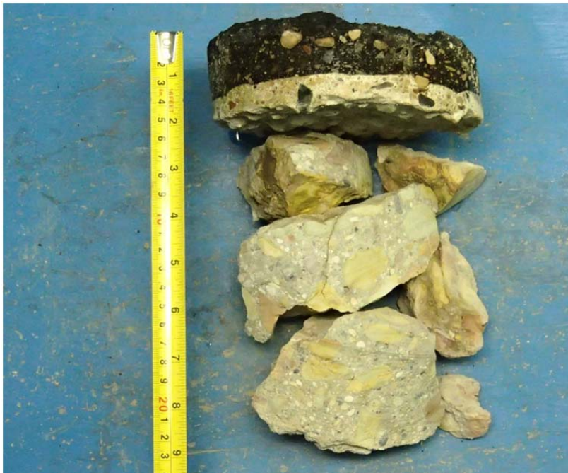
Core sample from Testhole TH2
