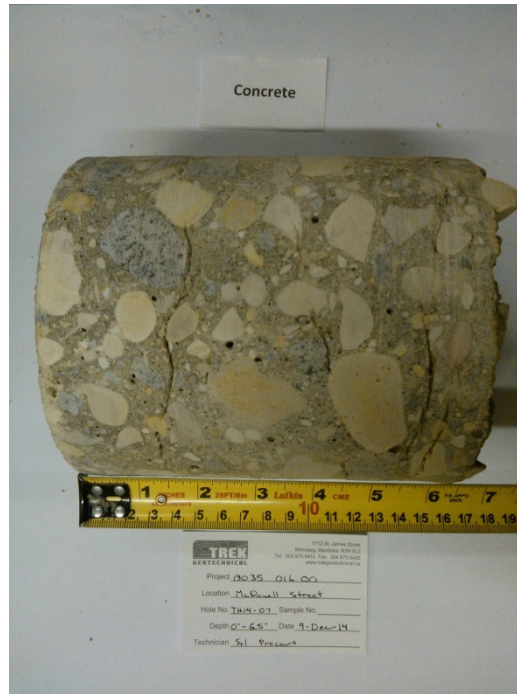
Photo 7: Concrete Core Sample From Test Hole TH14-07
