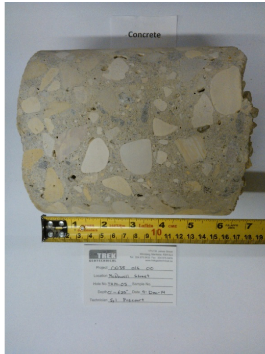
Photo 5: Concrete Core Sample From Test Hole TH14-05
