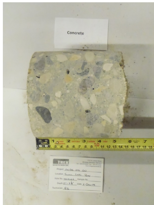
Photo 6: Concrete Core Sample From Test Hole TH14-06
