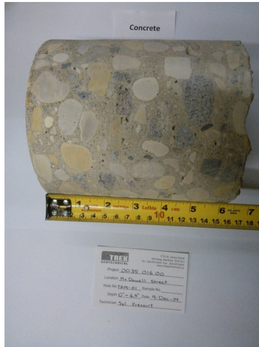
Photo 1: Concrete Core Sample From Test Hole TH14-01
