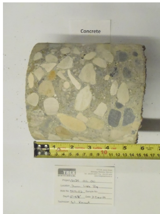
Photo 2: Concrete Core Sample From Test Hole TH14-02
