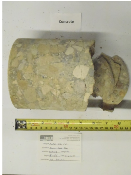
Photo 3: Concrete Core Sample From Test Hole TH14-03
