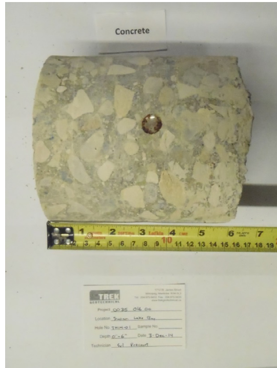
Photo 1: Concrete Core Sample From Test Hole TH14-01
