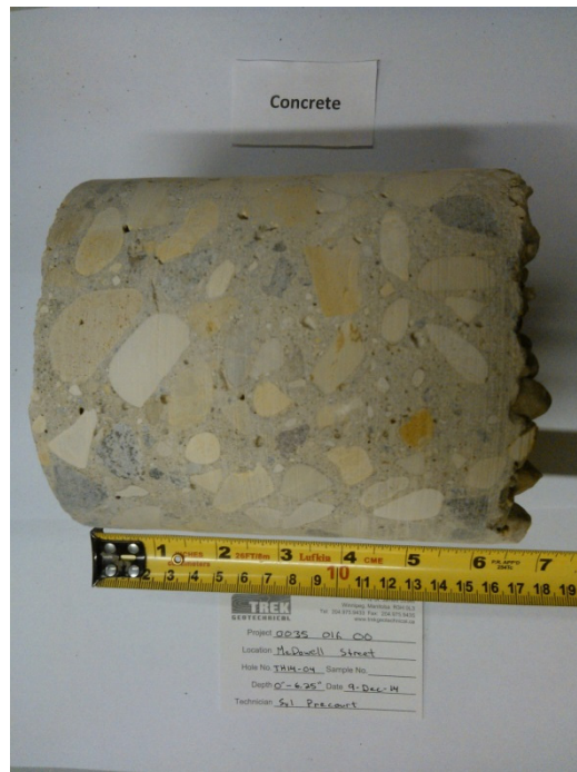
Photo 4: Concrete Core Sample From Test Hole TH14-04
