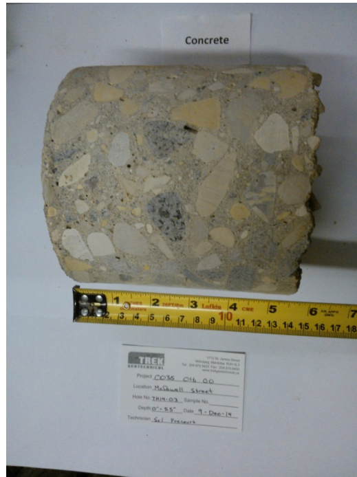
Photo 3: Concrete Core Sample From Test Hole TH14-03
