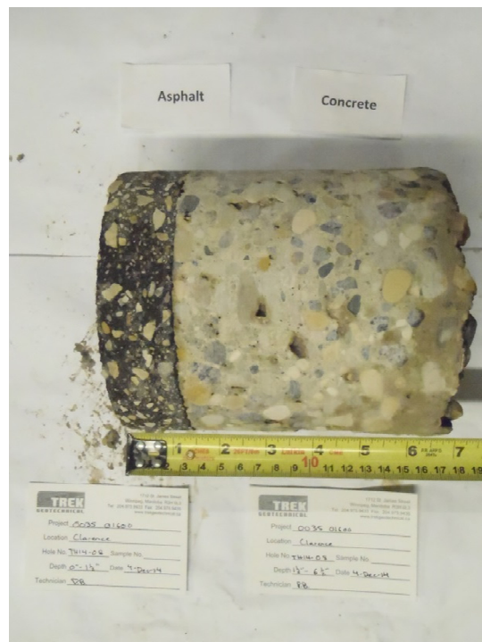
Photo 8: Concrete Core Sample From Test Hole TH14-08
