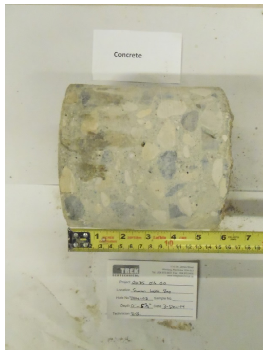
Photo 8: Concrete Core Sample From Test Hole TH14-08
