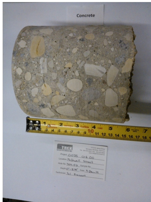
Photo 2: Concrete Core Sample From Test Hole TH14-02
