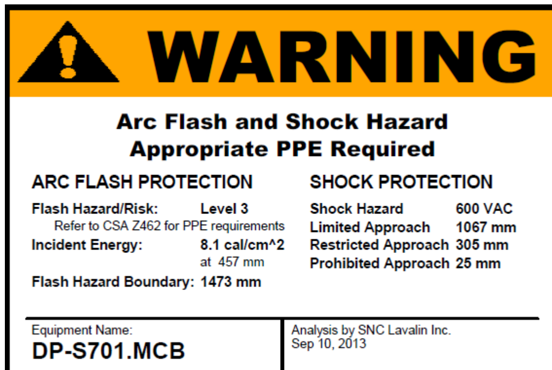
Figure 12-2 : Arc Flash Warning Label, Category 0 through 4 - Large
