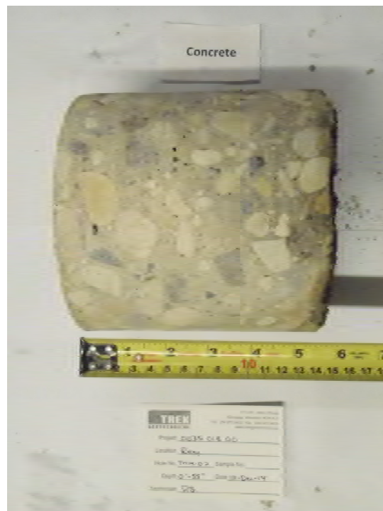
Photo 2: Concrete Core Sample From Test Hole TH14-02
