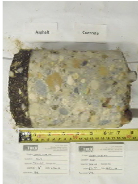
Photo 7: Concrete Core Sample From Test Hole TH14-07
