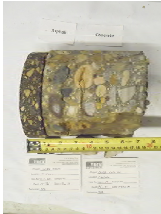
Photo 3: Concrete Core Sample From Test Hole TH14-03
