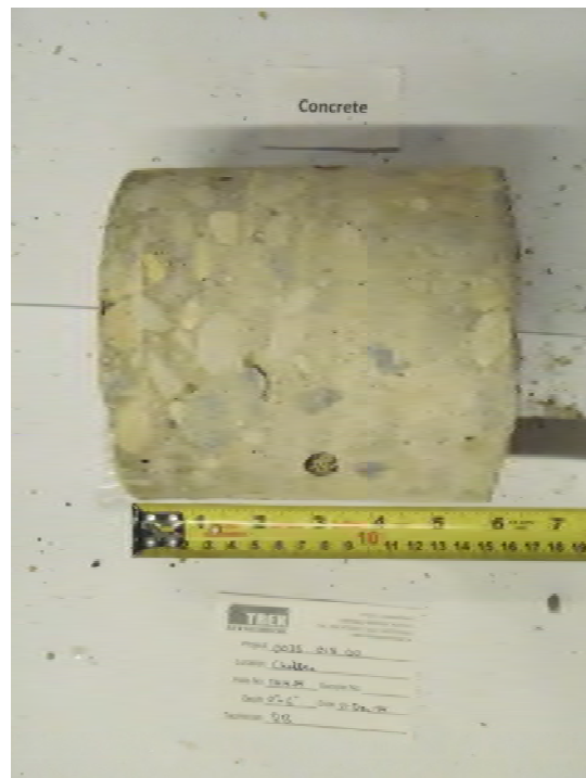
Photo 4: Concrete Core Sample From Test Hole TH14-04
