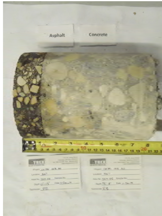
Photo 5: Concrete Core Sample From Test Hole TH14-05
