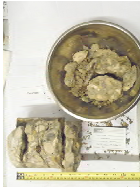
Photo 5: Concrete Core Sample From Test Hole TH14-05
