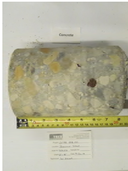
Photo 2: Concrete Core Sample From Test Hole TH14-02
