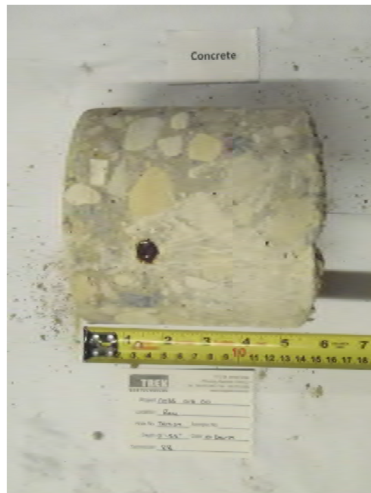
Photo 4: Concrete Core Sample From Test Hole TH14-04
