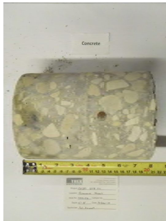
Photo 6: Concrete Core Sample From Test Hole TH14-06
