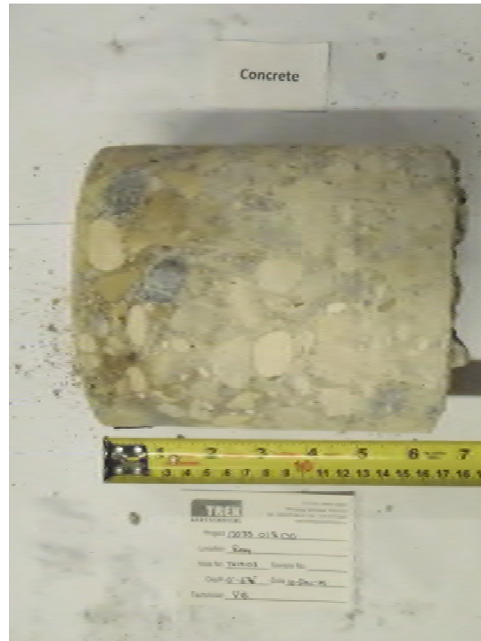
Photo 3: Concrete Core Sample From Test Hole TH14-03
