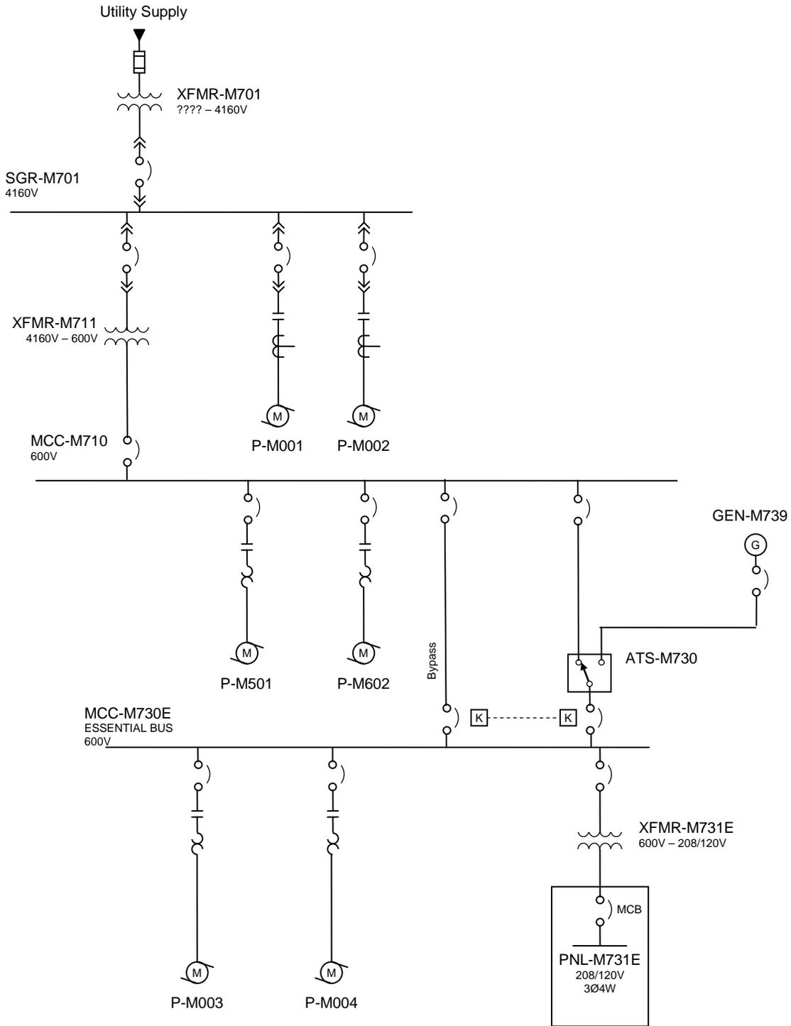
**Figure 3-8: Configuration H - MV Distribution with Essential Bus**
