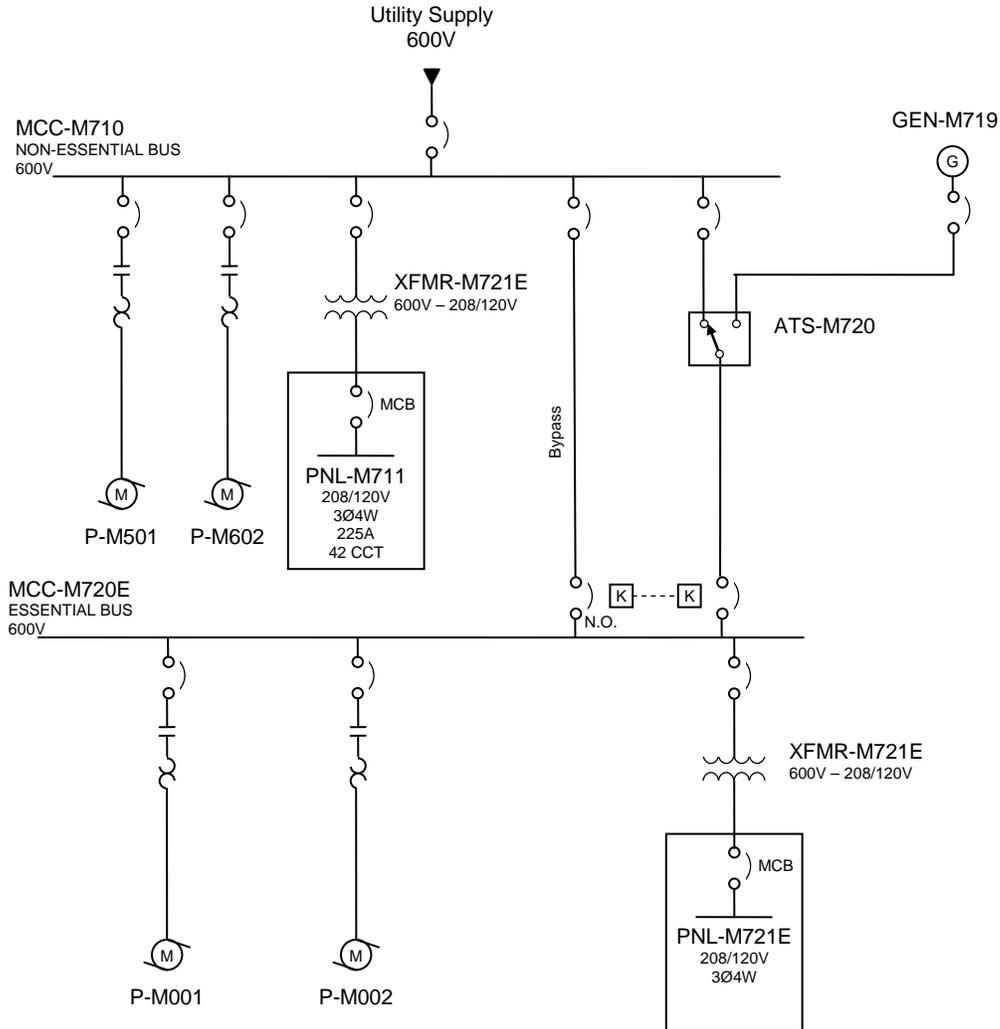
**Figure 3-5: Configuration E - 600V Distribution with Essential Bus**
