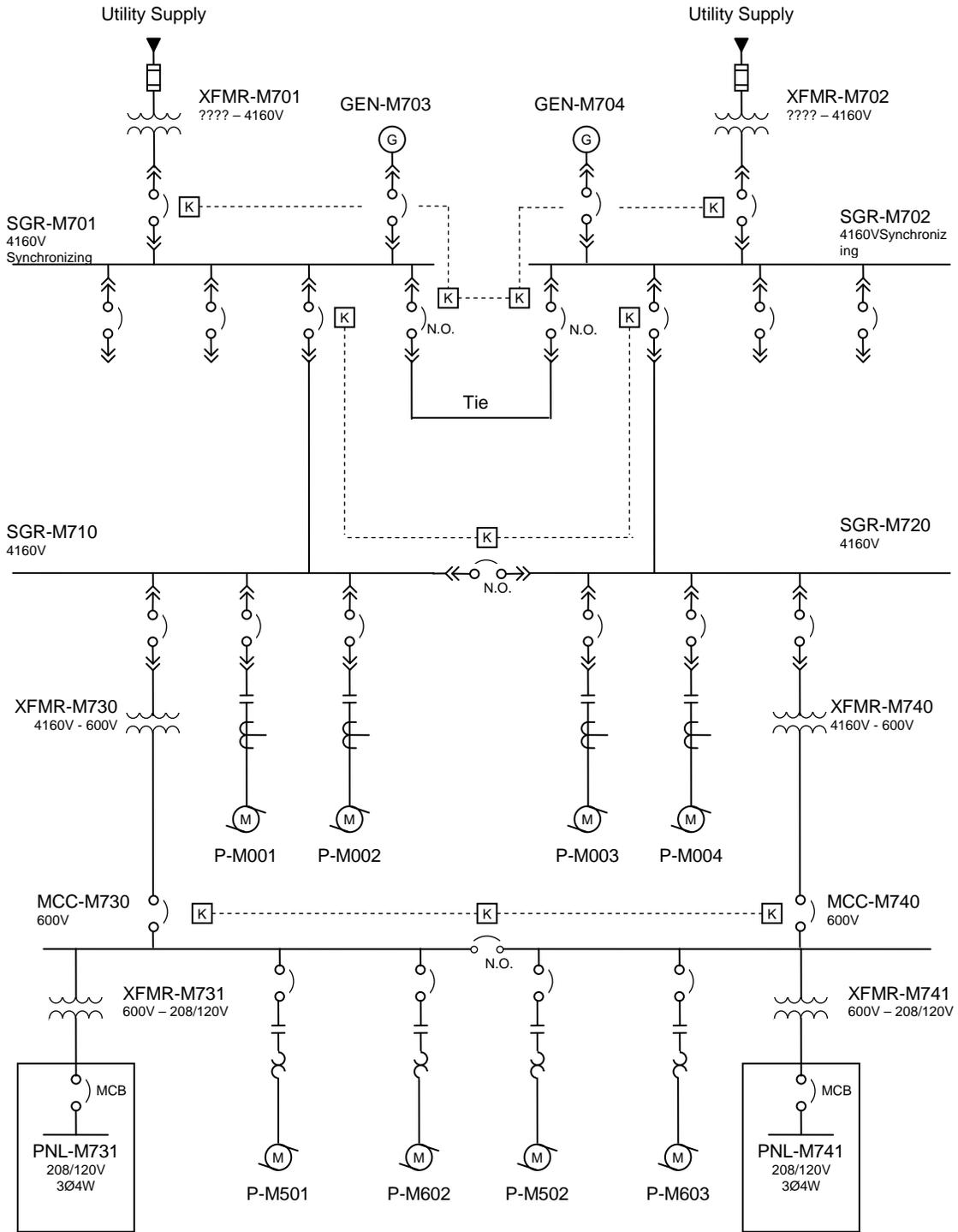
**Figure 3-10: Configuration J - MV Redundant with Integrated Generation**
