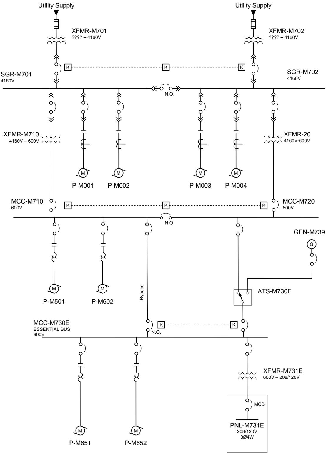
**Figure 3-9: Configuration I - MV Redundant with Essential Bus**
