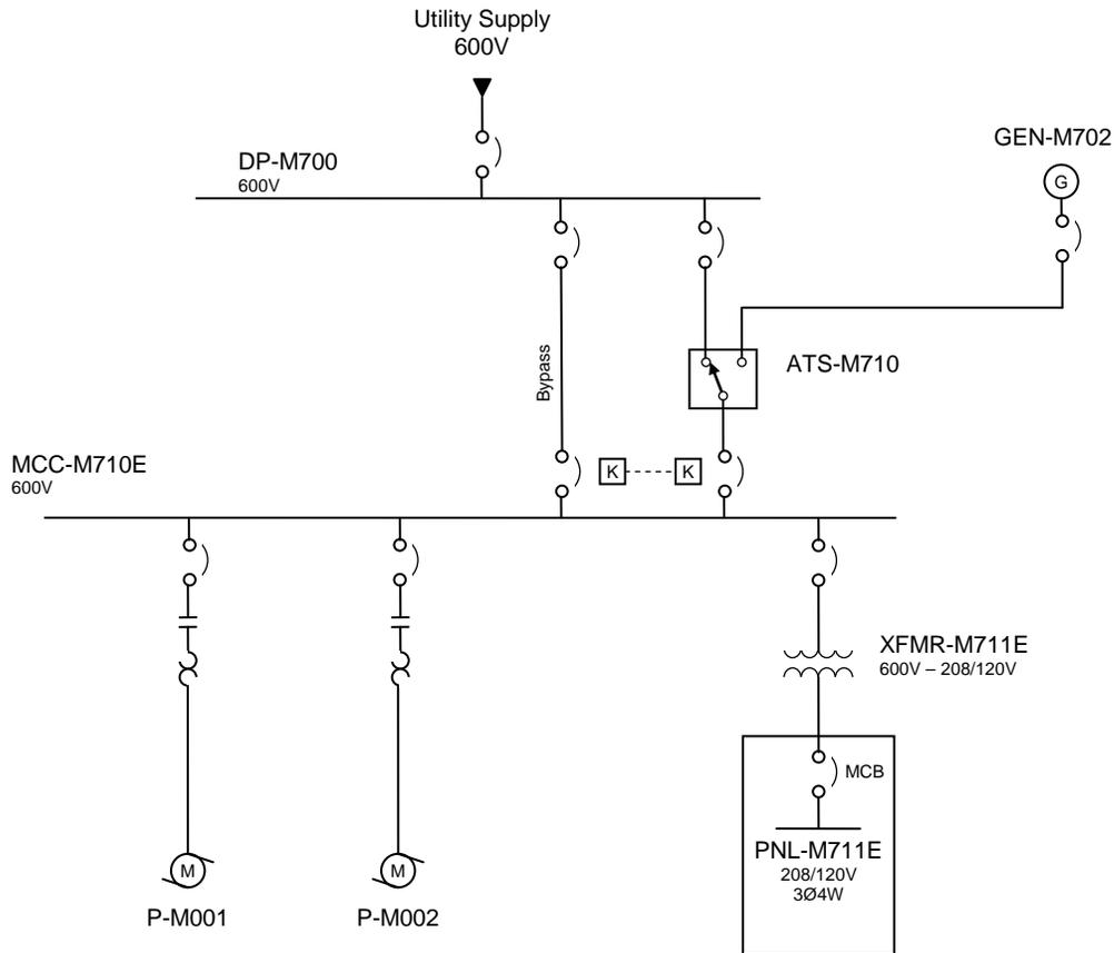
**Figure 3-4: Configuration D - 600V Distribution with Standby Generator**
