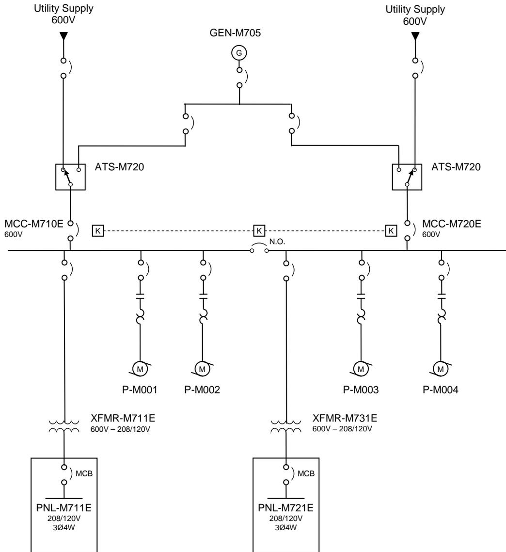
**Figure 3-6: Configuration F - 600V Redundant with Standby Generator**
