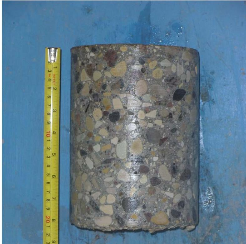
Core sample from Testhole TH6
