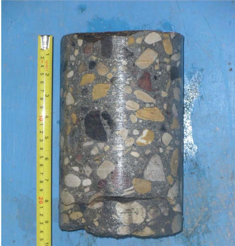
Core sample from Testhole TH3
