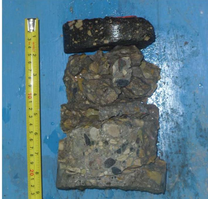
Core sample from Testhole TH3
