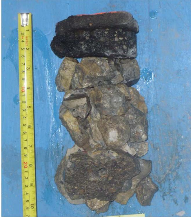
Core sample from Testhole TH1
