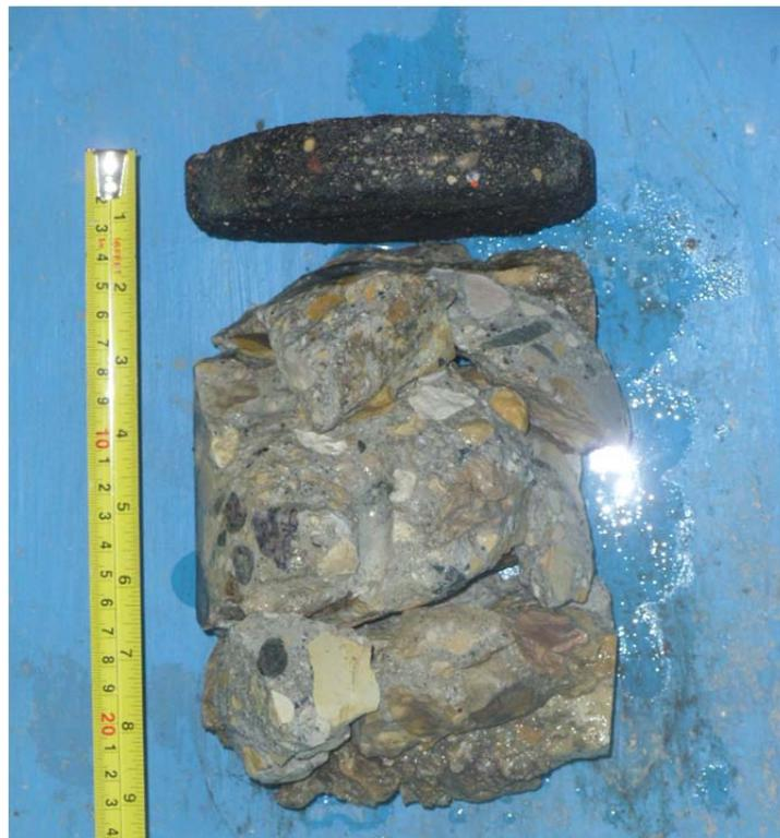
Core sample from Testhole TH4
