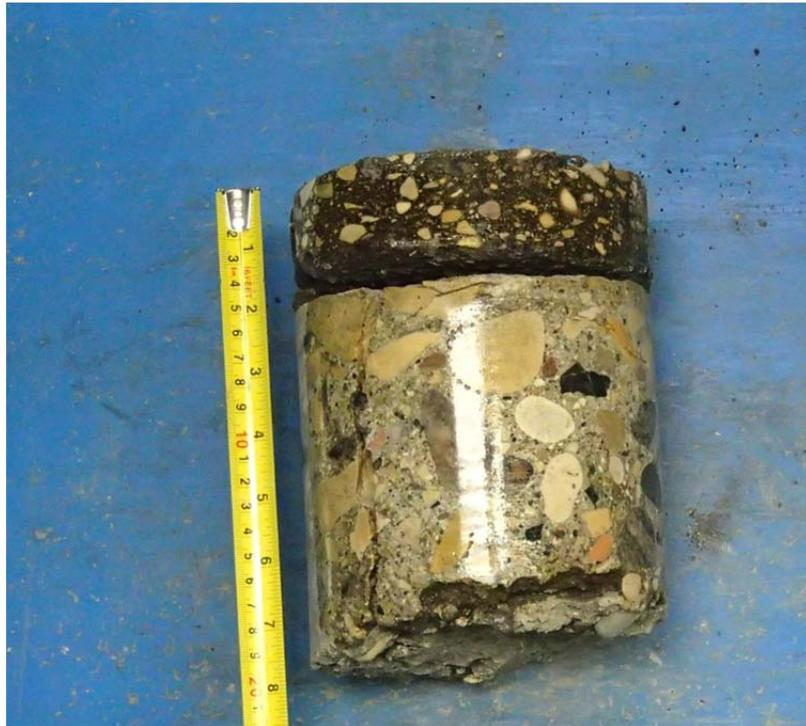
Core sample from Testhole TH4
