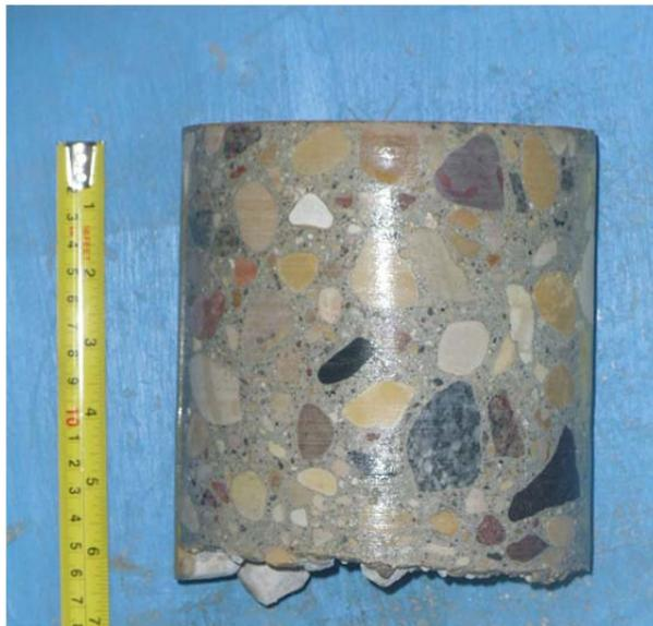
Core sample from Testhole TH2
