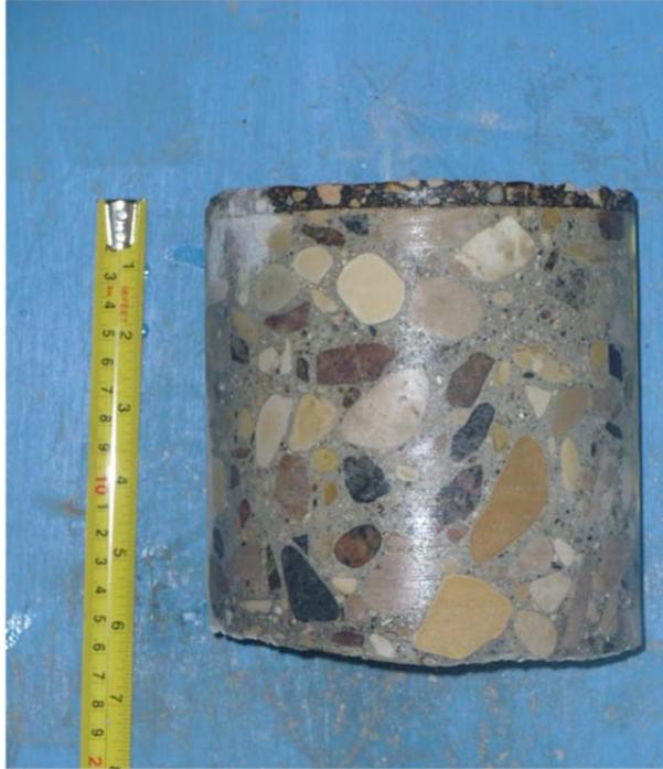
Core sample from Testhole TH3
