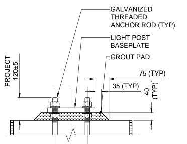
LIGHT POST ANCHORAGE INSTALLATION NOTES: CAST ANCHORS INTO CONCRETE PILE. SET ANCHOR ROD LOCATION AND PROJECTION TO THE TOLERANCES SHOWN ON THE DRAWINGS BY USE OF A PLYWOOD TEMPLATE. PROVIDE TEMPORARY HEAVY HEX NUTS TO HOLD THE ANCHORS TO THE TEMPLATE WITH THE CORRECT THREAD PROJECTION DURING THE CONCRETE POUR. DISCARD THESE NUTS FOLLOWING THE POUR AND PROVIDE THE NUTS SHOWN ON THE DRAWINGS FOR THE PERMANENT INSTALLATION.
