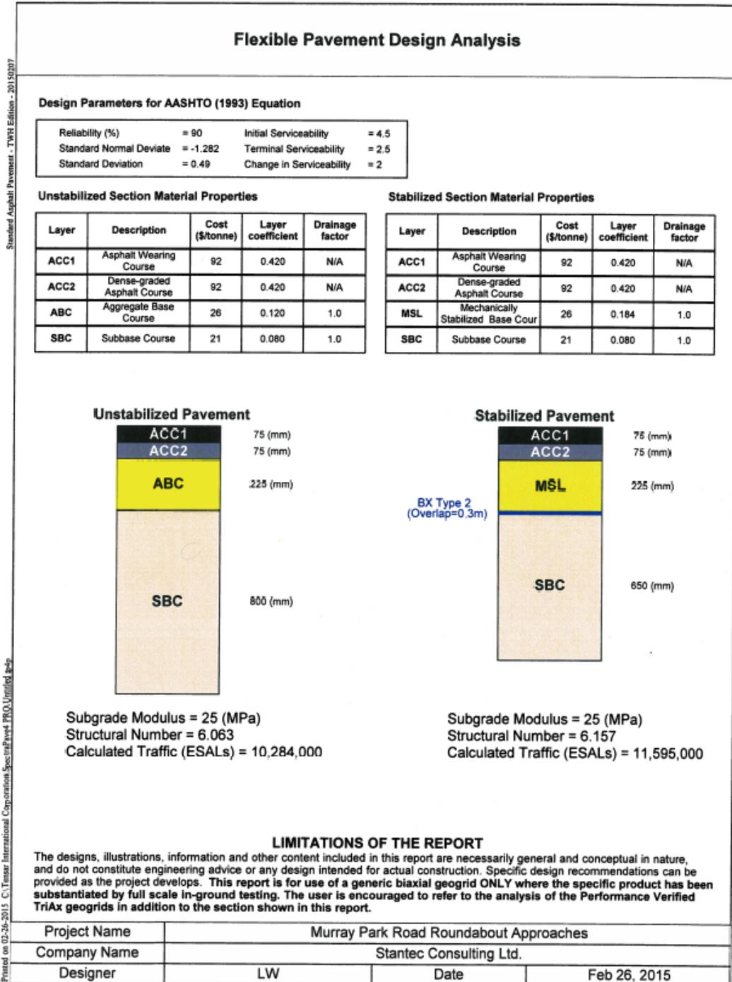
Figure A.7: SpectraPave Flexible Pavement Design Analysis with Geogrid for Murray Park Road Approaches – 25 Year Design Life
