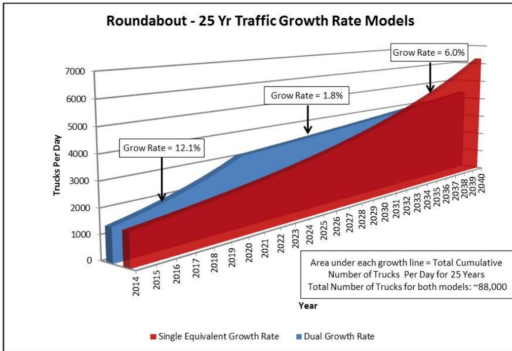
Figure 2: Sturgeon Rd & Murray Park Rd Roundabout, 25 Year Traffic Growth Rate Models
