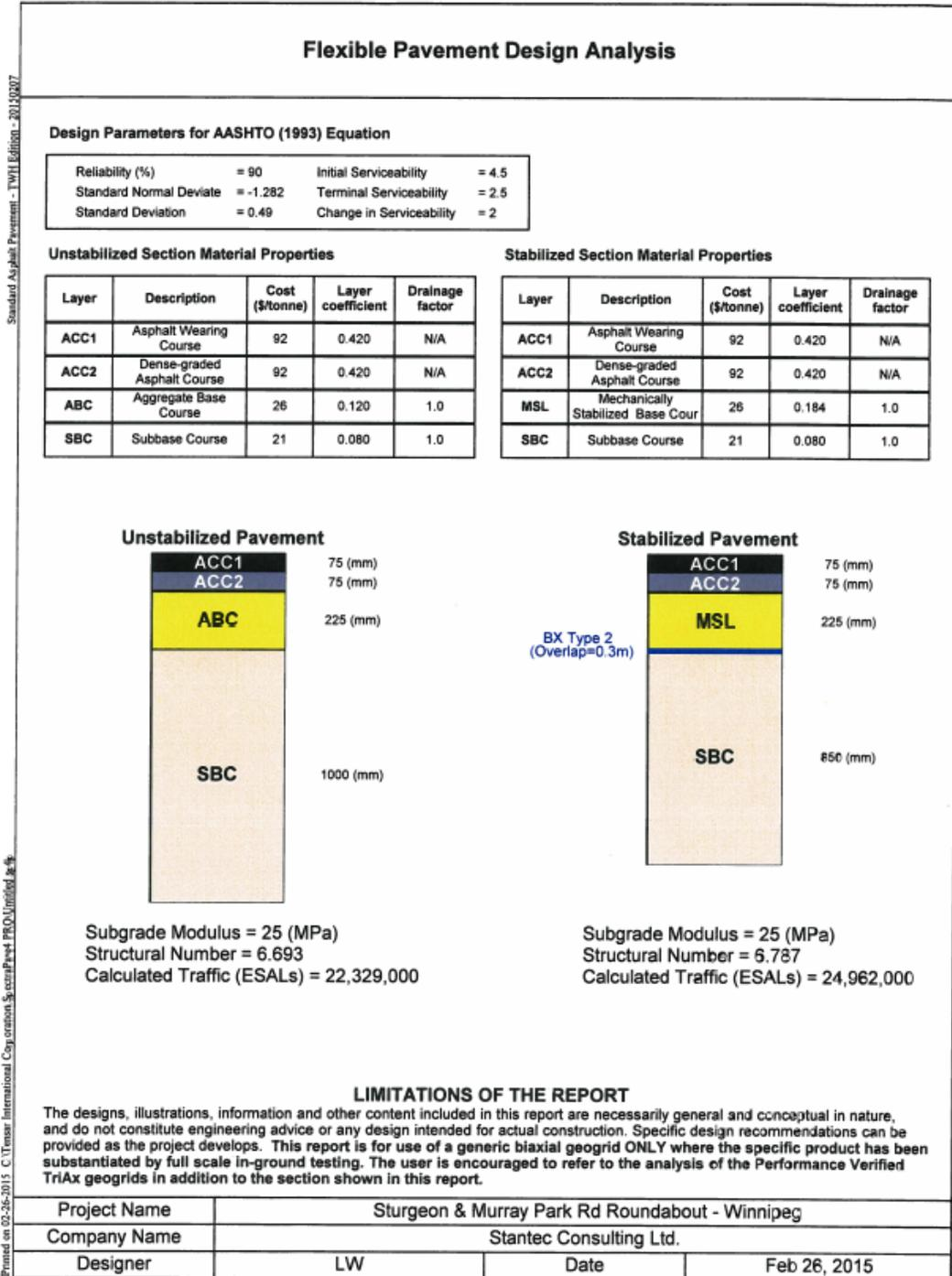
Figure A.5: SpectraPave Flexible Pavement Design Analysis with Geogrid for Roundabout – 25 Year Design Life
