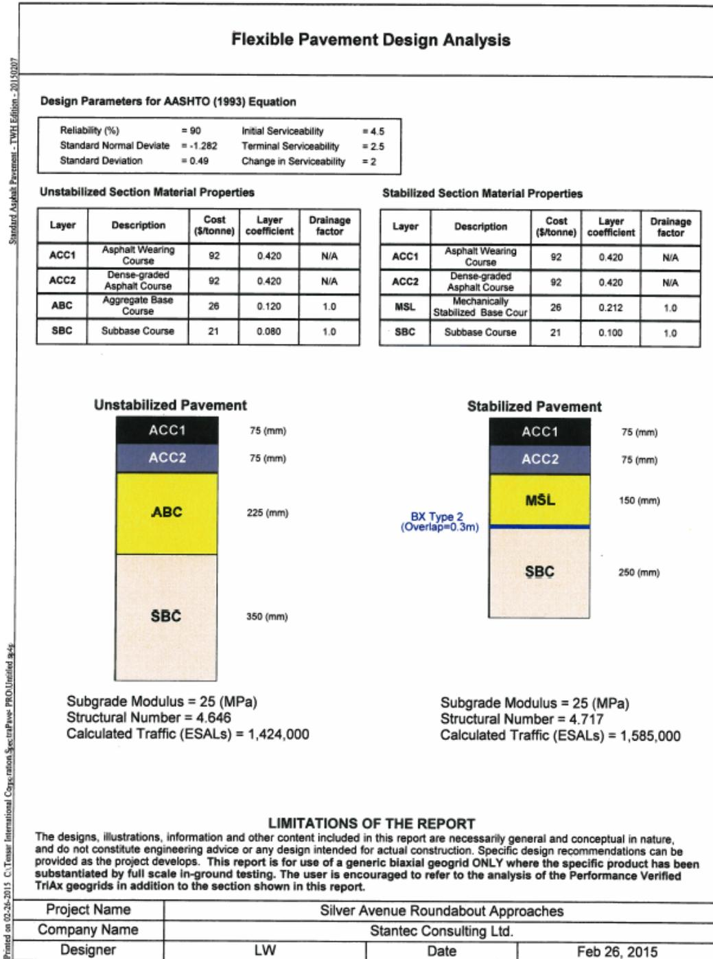
Figure A.8: SpectraPave Flexible Pavement Design Analysis with Geogrid for Silver Avenue Approach – 25 Year Design Life
