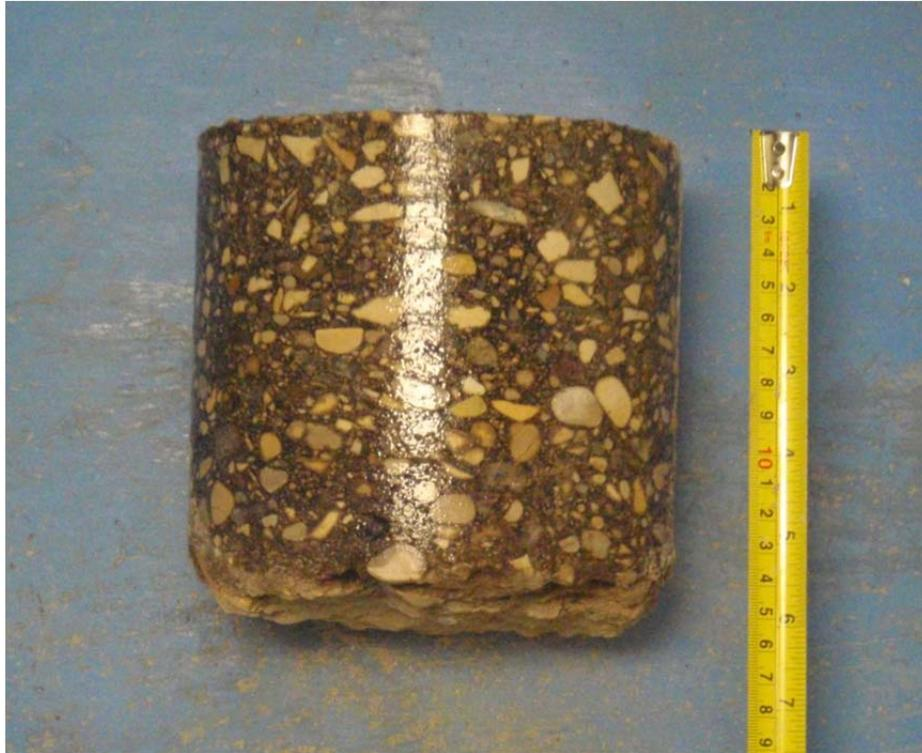
Core sample from Testhole TH3
