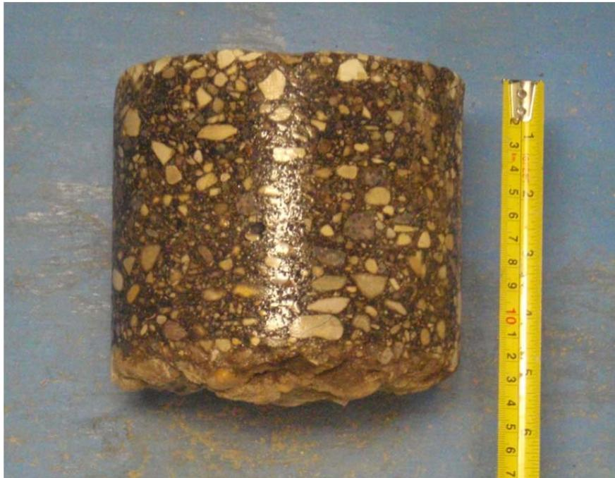
Core sample from Testhole TH2
