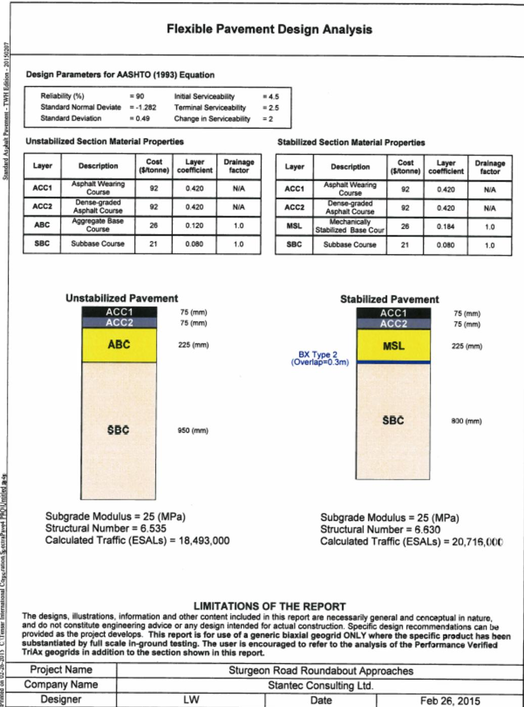
Figure A.6: SpectraPave Flexible Pavement Design Analysis with Geogrid for Sturgeon Road Approaches – 25 Year Design Life
