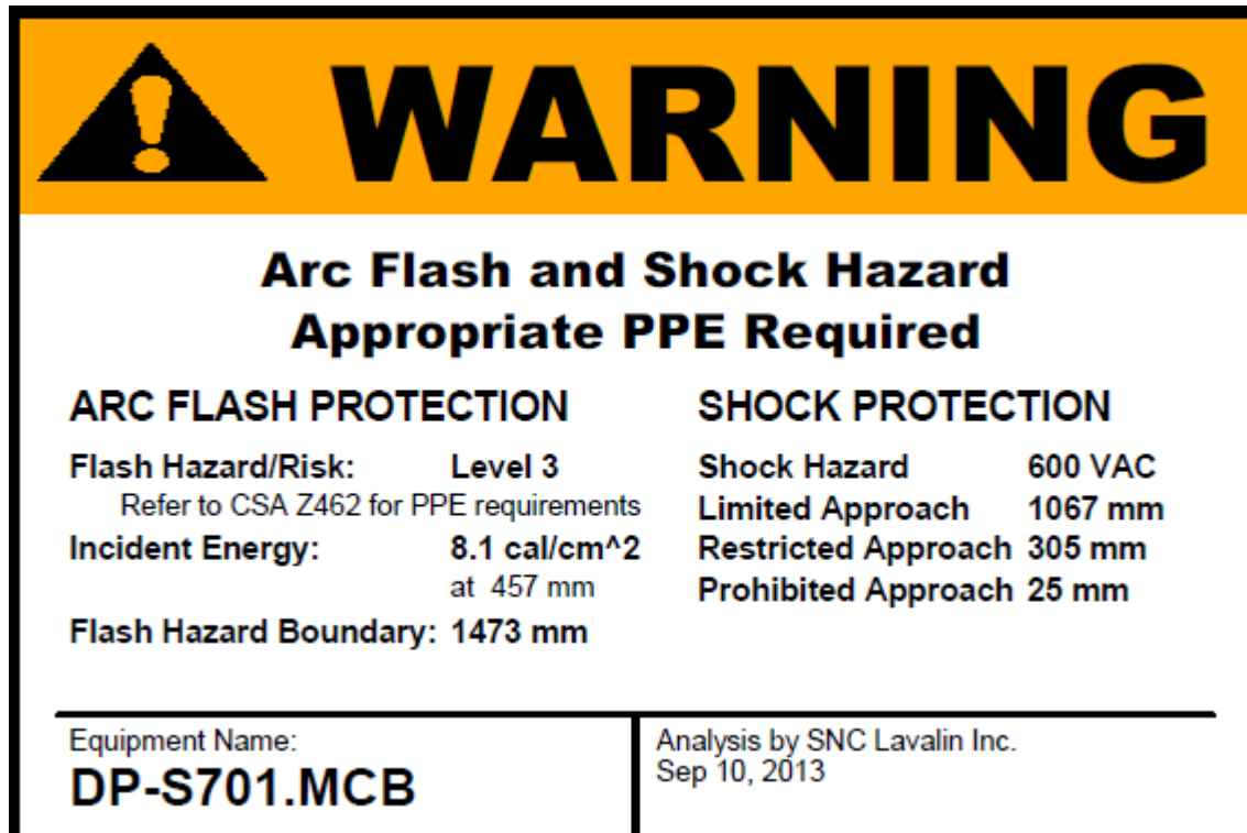
Figure 12-2 : Arc Flash Warning Label, Category 0 through 4 - Large
