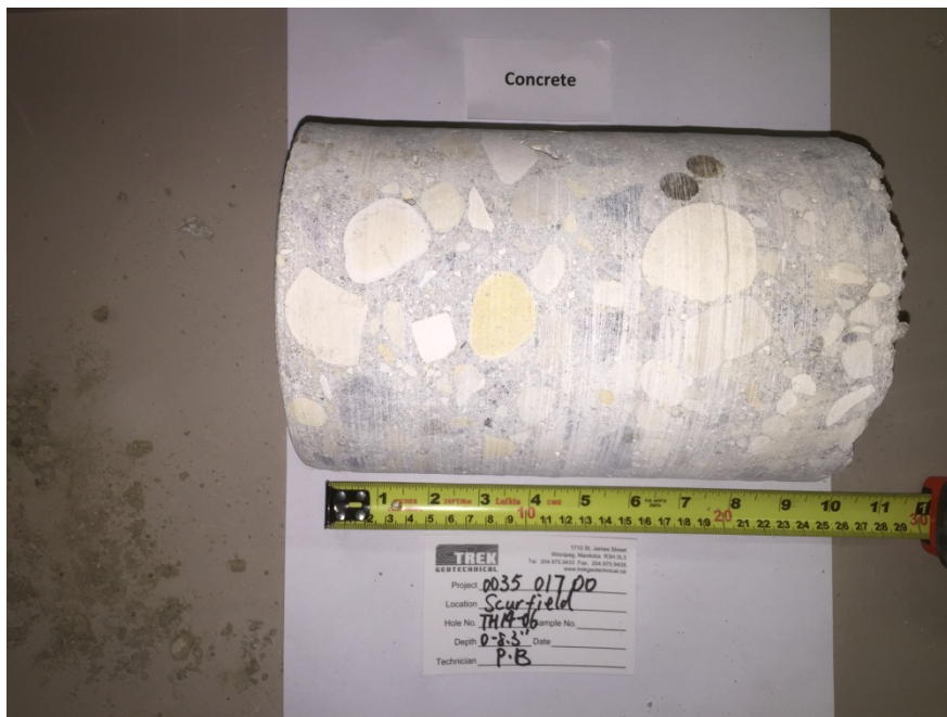
Photo 6: Concrete Core Sample From Test Hole TH14-06
