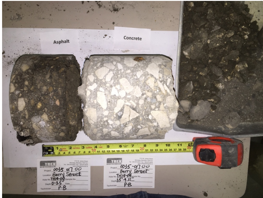
Photo 5: Concrete Core Sample From Test Hole TH14-04
