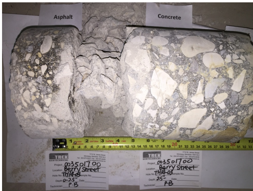
Photo 4: Concrete Core Sample From Test Hole TH14-03
