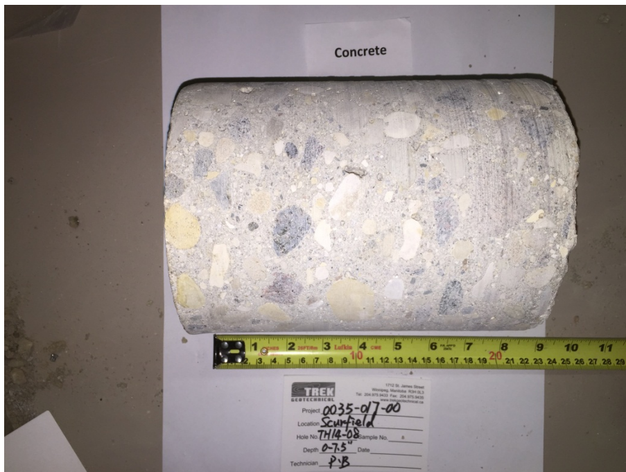
Photo 8: Concrete Core Sample From Test Hole TH14-08
