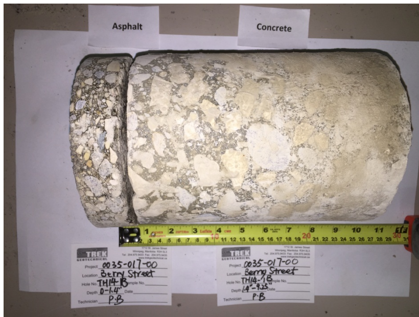
Photo 2: Concrete Core Sample From Test Hole TH14-01B
