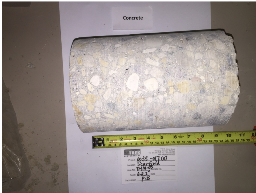
Photo 5: Concrete Core Sample From Test Hole TH14-05
