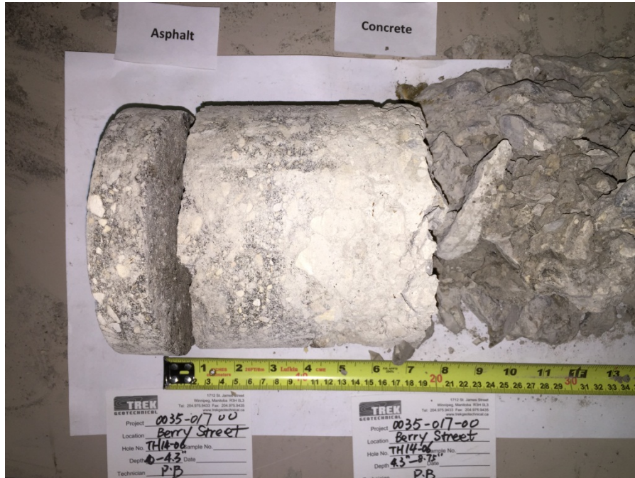
Photo 7: Concrete Core Sample From Test Hole TH14-06
