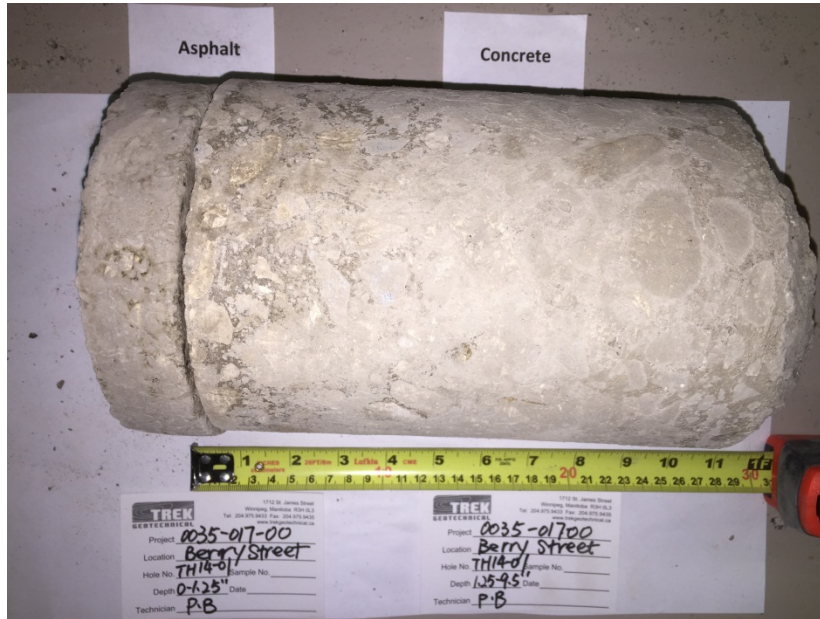
Photo 1: Concrete Core Sample From Test Hole TH14-01
