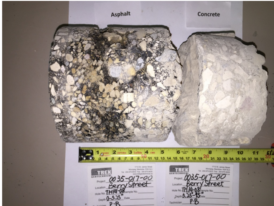
Photo 9: Concrete Core Sample From Test Hole TH14-08
