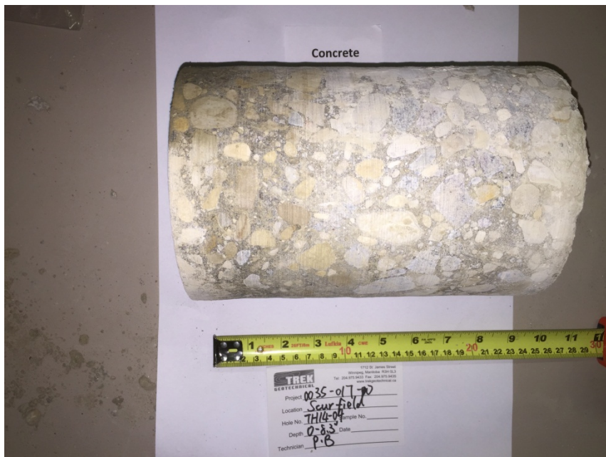
Photo 4: Concrete Core Sample From Test Hole TH14-4
