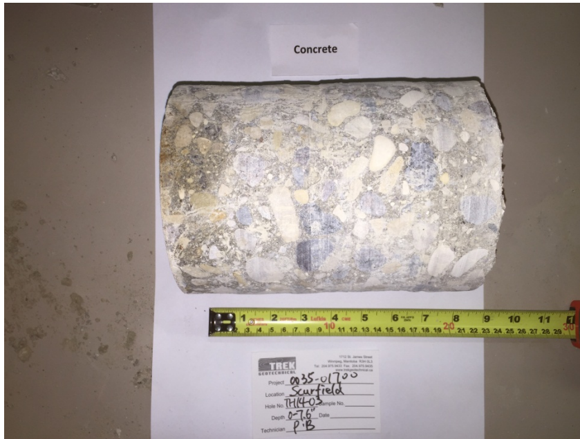
Photo 3: Concrete Core Sample From Test Hole TH14-03
