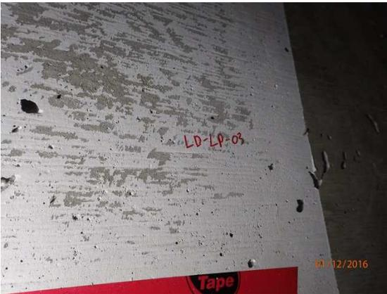
Photo 3. White non-lead-based paint on wall (Sample ID: LD-LP-03).
