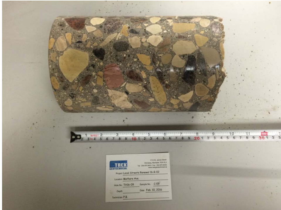
Photo 9: Concrete Core Sample From Test Hole TH15-09
