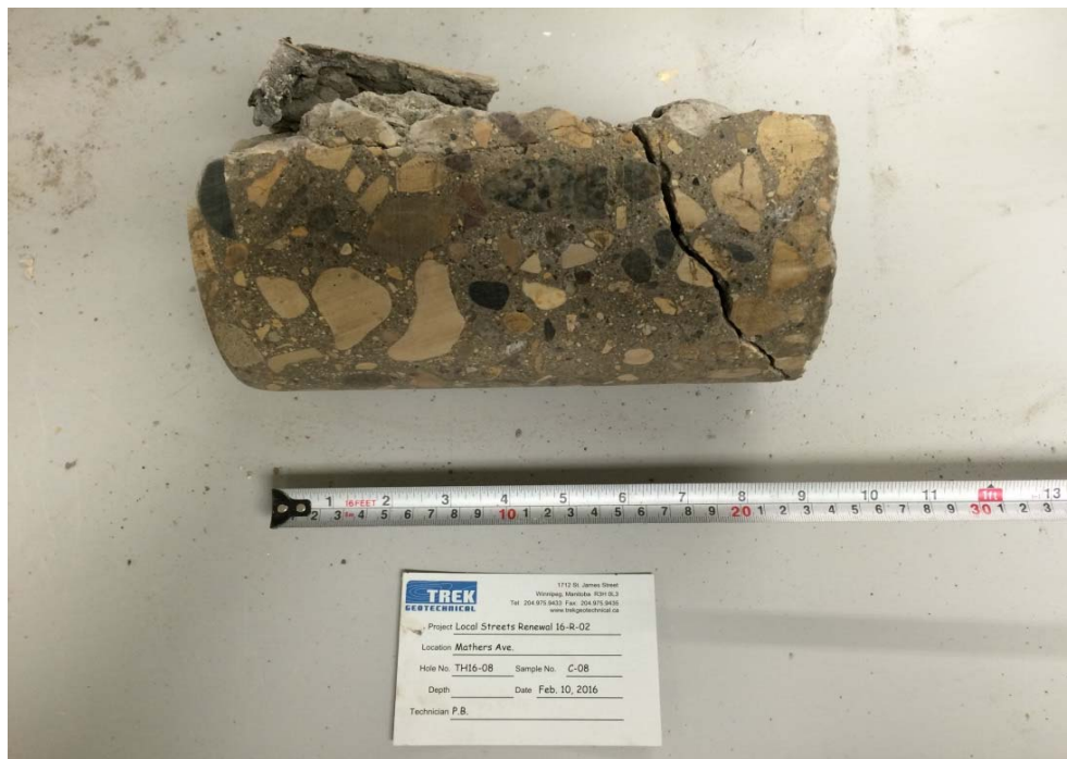
Photo 8: Pavement Core Sample at Test Hole TH16-08
