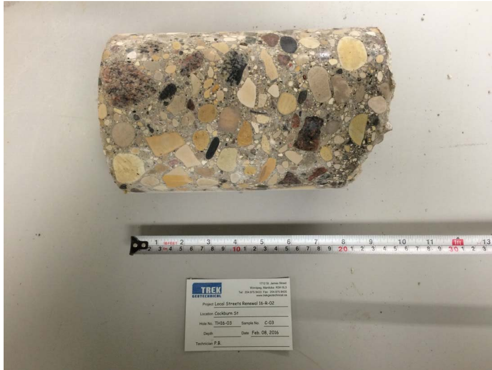
Photo 3: Pavement Core Sample at Test Hole TH16-03
