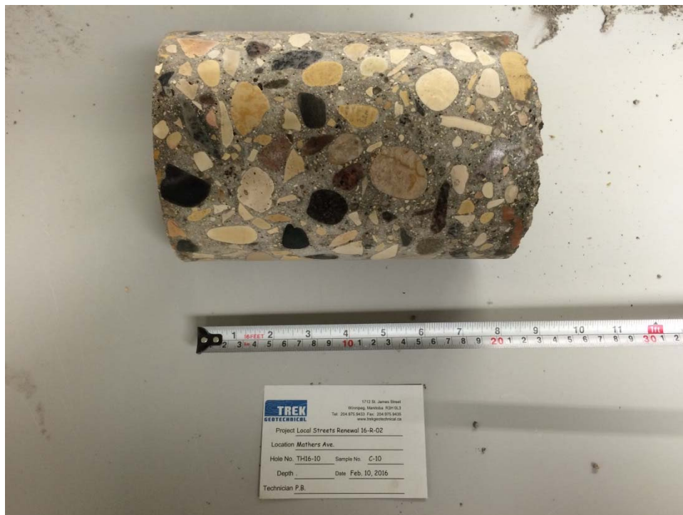
Photo 10: Concrete Core Sample From Test Hole TH15-10
