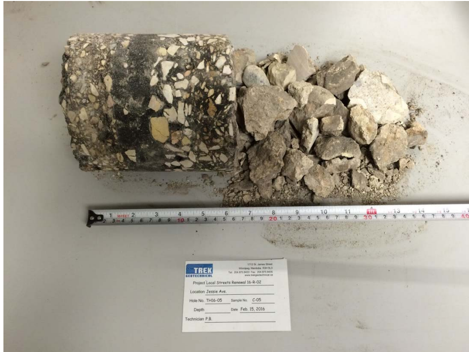
Photo 5: Pavement Core Sample at Test Hole TH16-05
