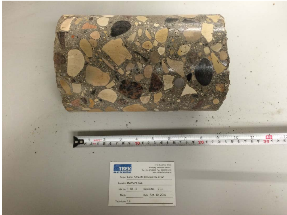
Photo 11: Concrete Core Sample From Test Hole TH15-11
