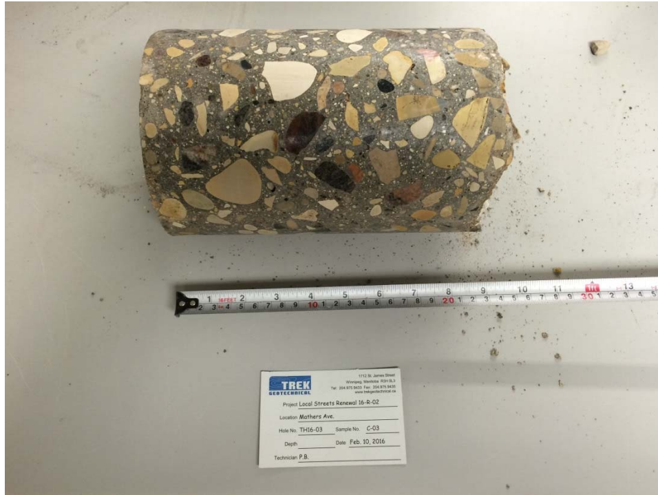
Photo 3: Pavement Core Sample at Test Hole TH16-03
