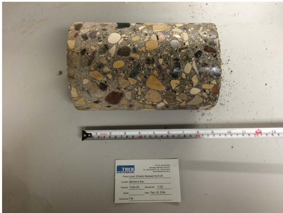
Photo 2: Pavement Core Sample at Test Hole TH16-02
