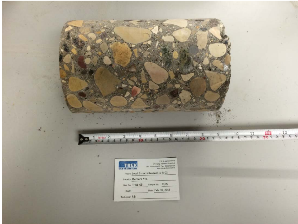
Photo 5: Pavement Core Sample at Test Hole TH16-05
