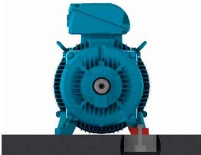
Figure 6-3 – Motor installed on concrete base
