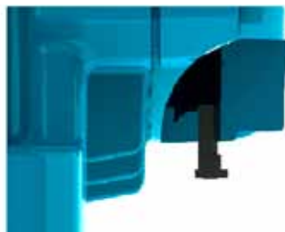
Figure 6-1 – Detail of the rubber drain plug mounted in open position
