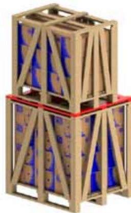
Figure 5-5 – Use of additional battens for stacking
