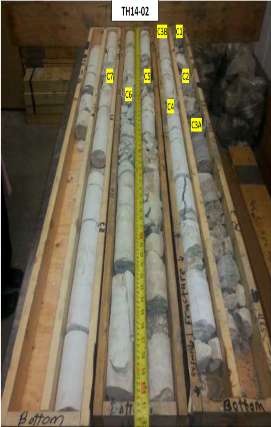
Figure 03a – Rock cores from (TH14-02) – Preliminary design stage
