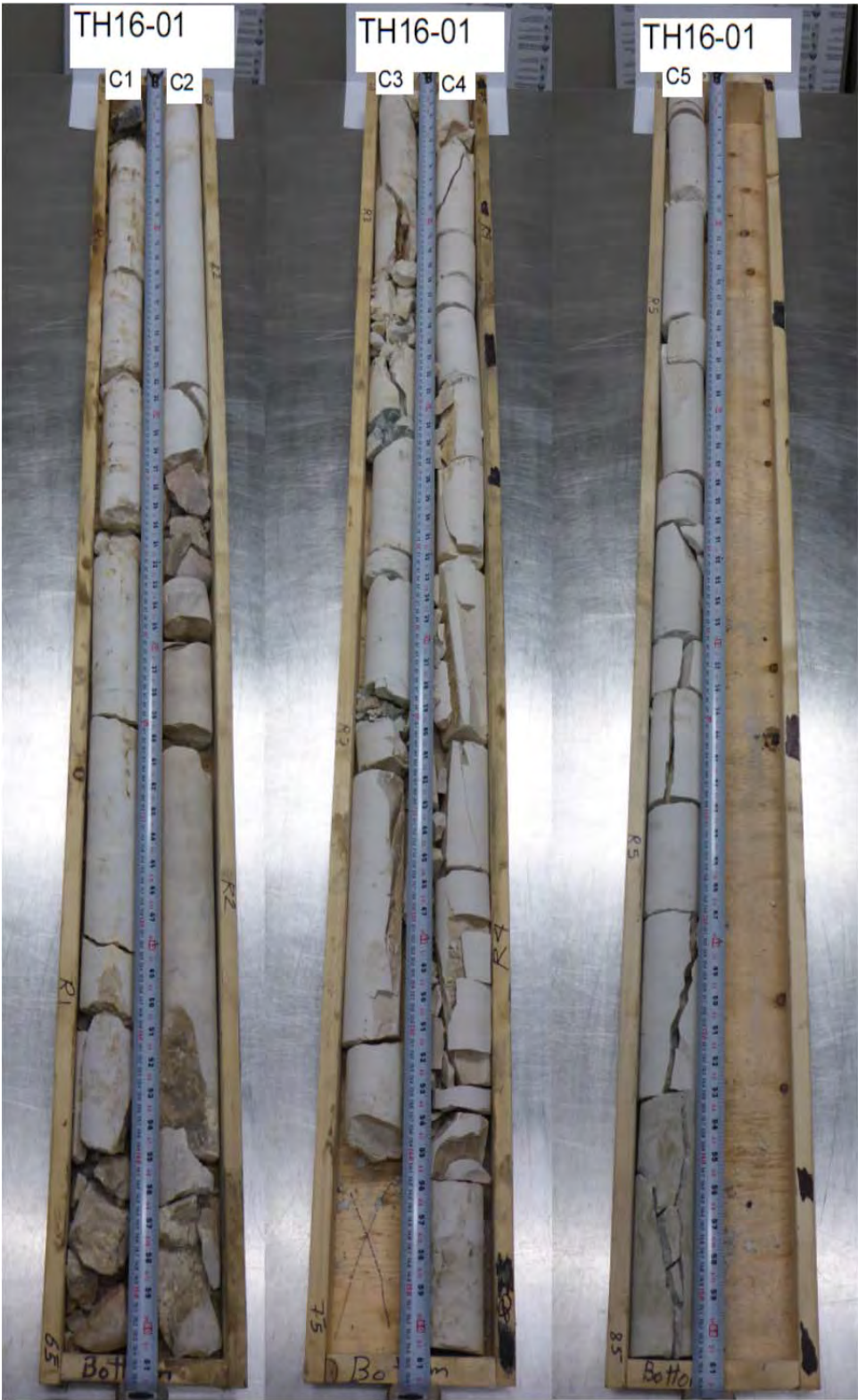
Figure 02a – Rock cores from (TH 16-01) – Detailed design stage
