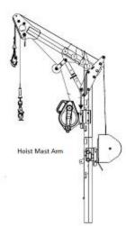
6.23 Location: will be mounted in driver's side rear cargo area. Exact mounting locations of hooks and floor sleeve TBD at the time of outfitting.
