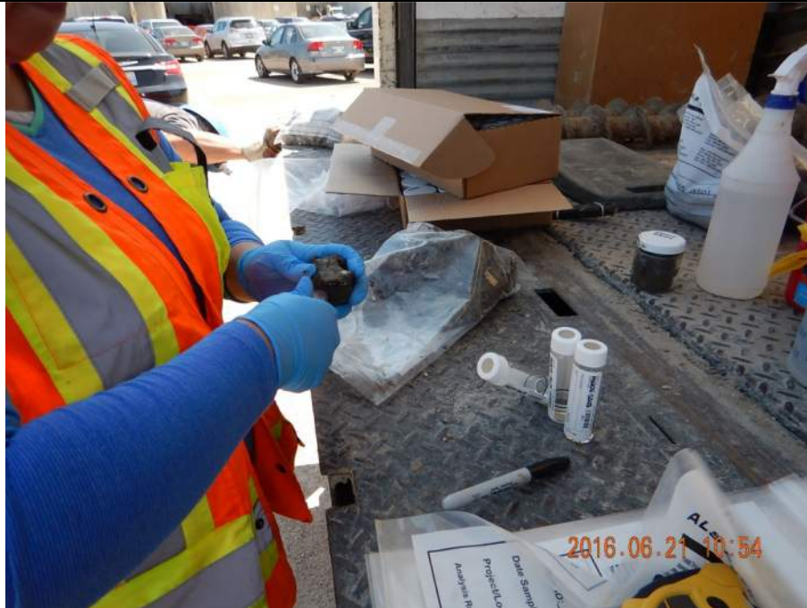
Photo 3. Extracting sample core for in-field methanol preservation.
