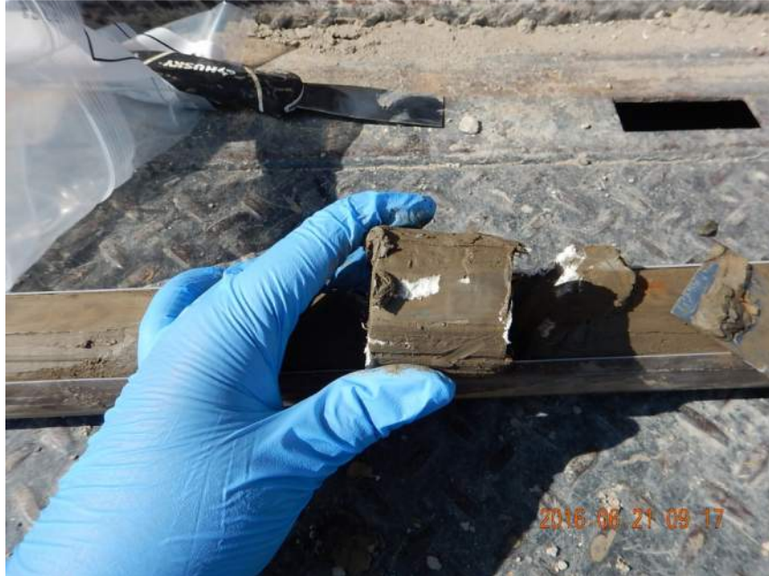
Photo 1. Representative photo of Silty clay with gypsum nodule unit found throughout the Site while drilling.
