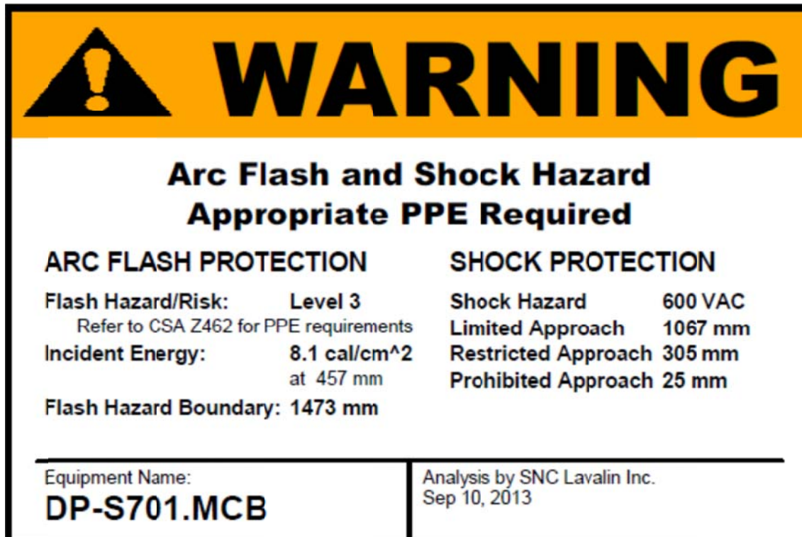
Figure 13-2 : Arc Flash Warning Label, Category 0 through 4 - Large
