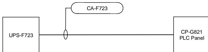
Figure 7-2: Instrument Cable Identification Example – Identified Equipment
