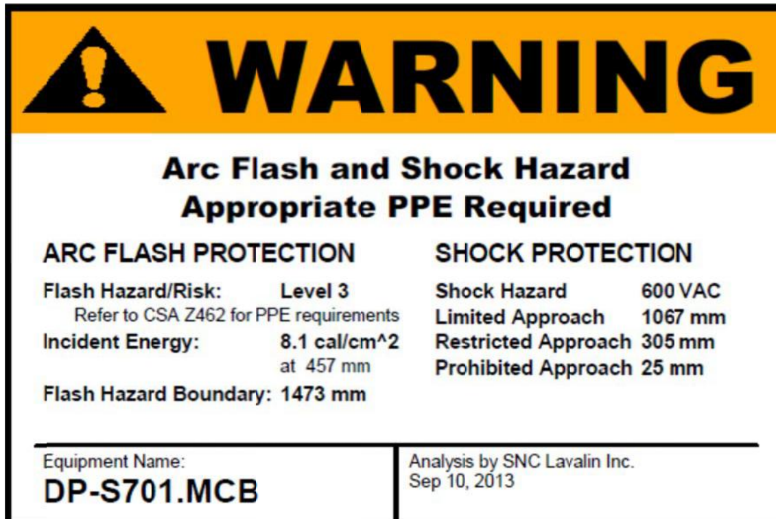
Figure 13-2 : Arc Flash Warning Label, Category 0 through 4 - Large
