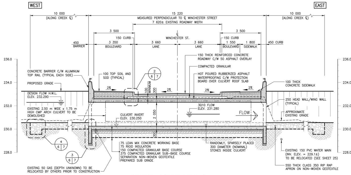
**SECTION PERPENDICULAR TO ROADWAY AT CULVERT**
