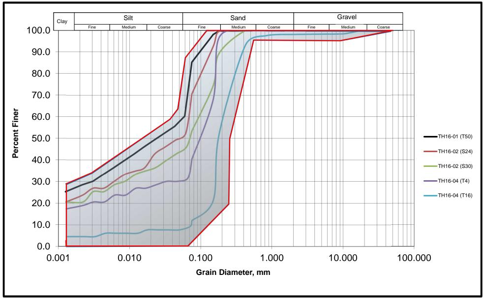
Figure C1: Baseline Grain Size Distribution Envelope for Alluvial Sand Soil Unit
