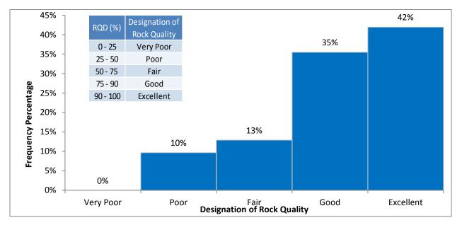
Figure 6-1: Histogram Distribution of RQD within Test holes
