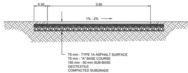
ASPHALT PATH TYPICAL CROSS SECTION
