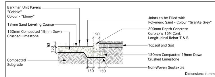
**4** UNIT PAVING AND EDGER CURB
