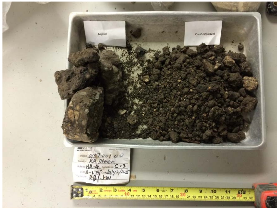
Photo 3: Asphalt Core Sample and underlying granular fill from Probe Hole PH15-03
