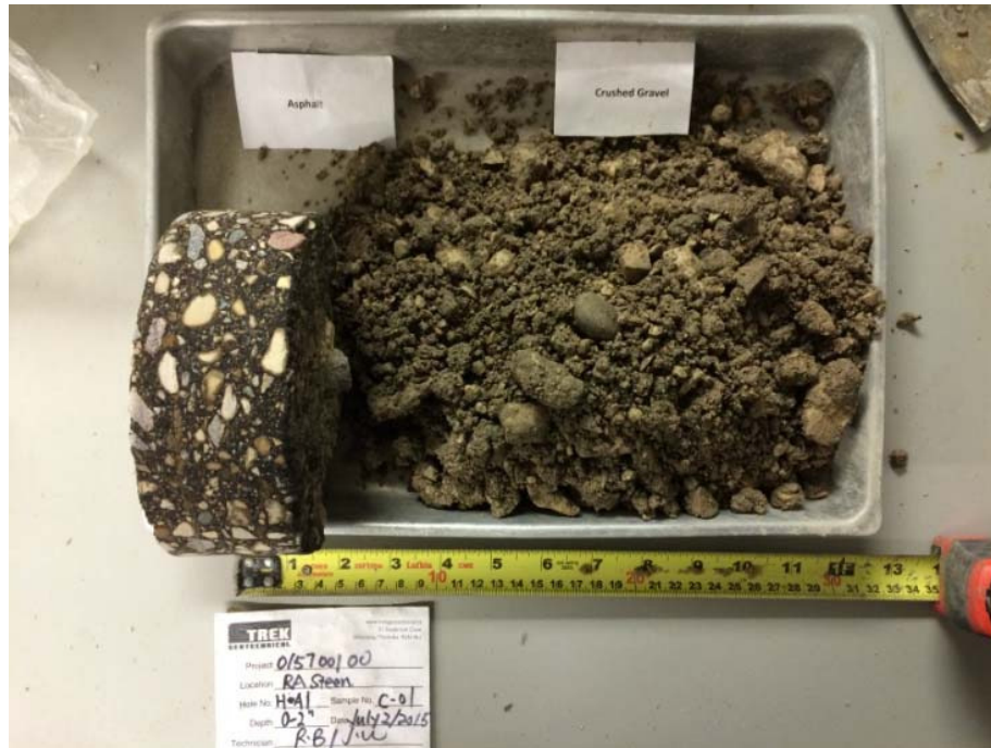
Photo 1: Asphalt Core Sample and underlying granular fill from Probe Hole PH15-01
