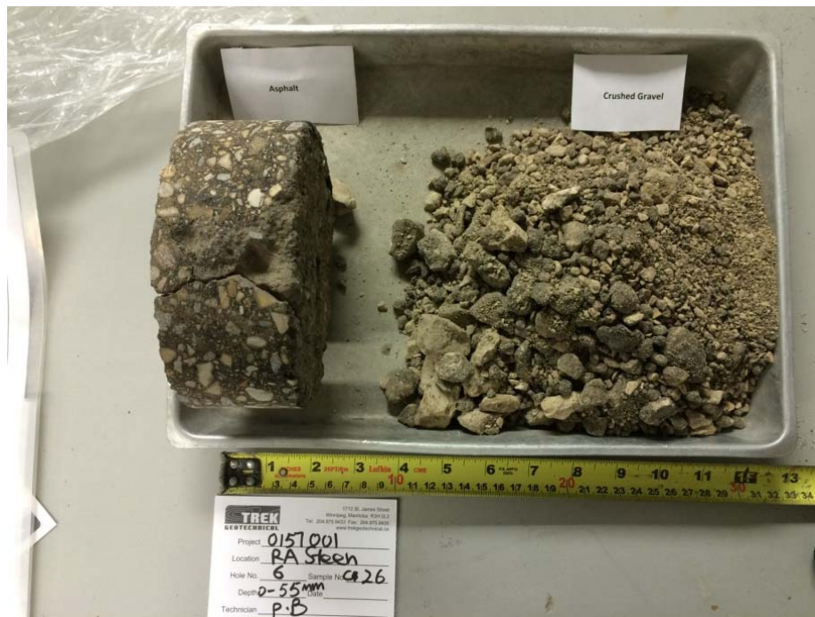
Photo 5: Asphalt Core Sample and underlying granular fill from Probe Hole PH15-05
