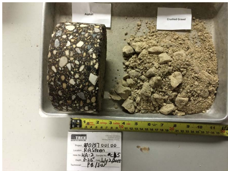
Photo 1: Asphalt Core Sample and underlying granular fill from Probe Hole PH15-01
