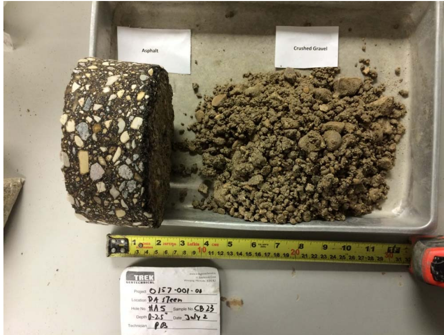
Photo 5: Asphalt Core Sample and underlying granular fill from Probe Hole PH15-05
