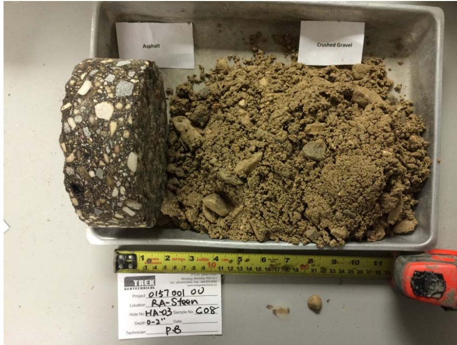
Photo 3: Asphalt Core Sample and underlying granular fill from Probe Hole PH15-03
