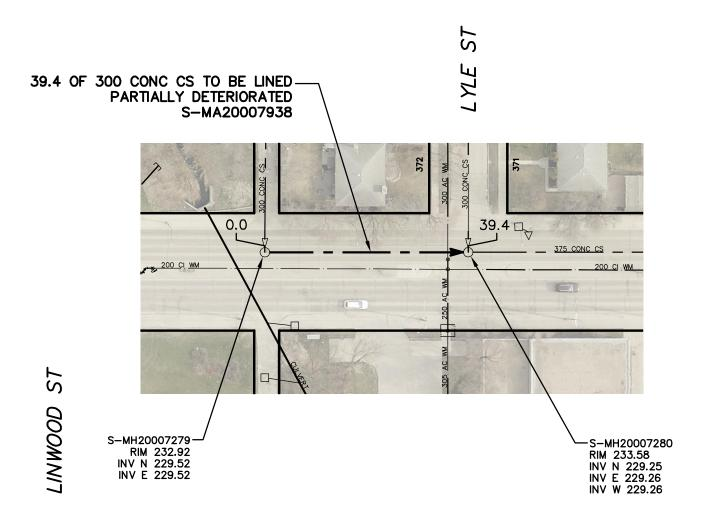
SEWER JUNCTION INFORMATION FROM SEWER VIDEO INSPECTION SEWER ID S-MA20007938 DISTANCE FROM MH ID S-MH20007279 DISTANCE DIAMETER CLOCK 100
