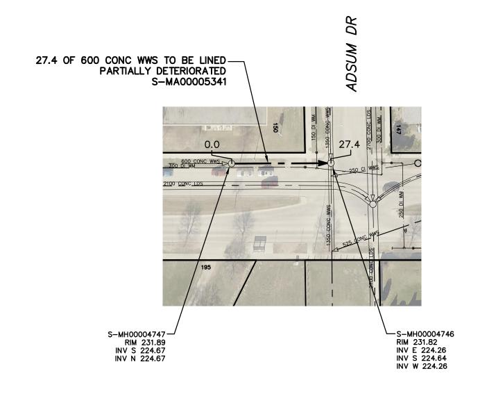
SEWER JUNCTION INFORMATION FROM SEWER VIDEO INSPECTION SEWER ID S-MA00005341 DISTANCE FROM MH ID S-MH00004747 DISTANCE DIAMETER CLOCK 13.3 150 10
