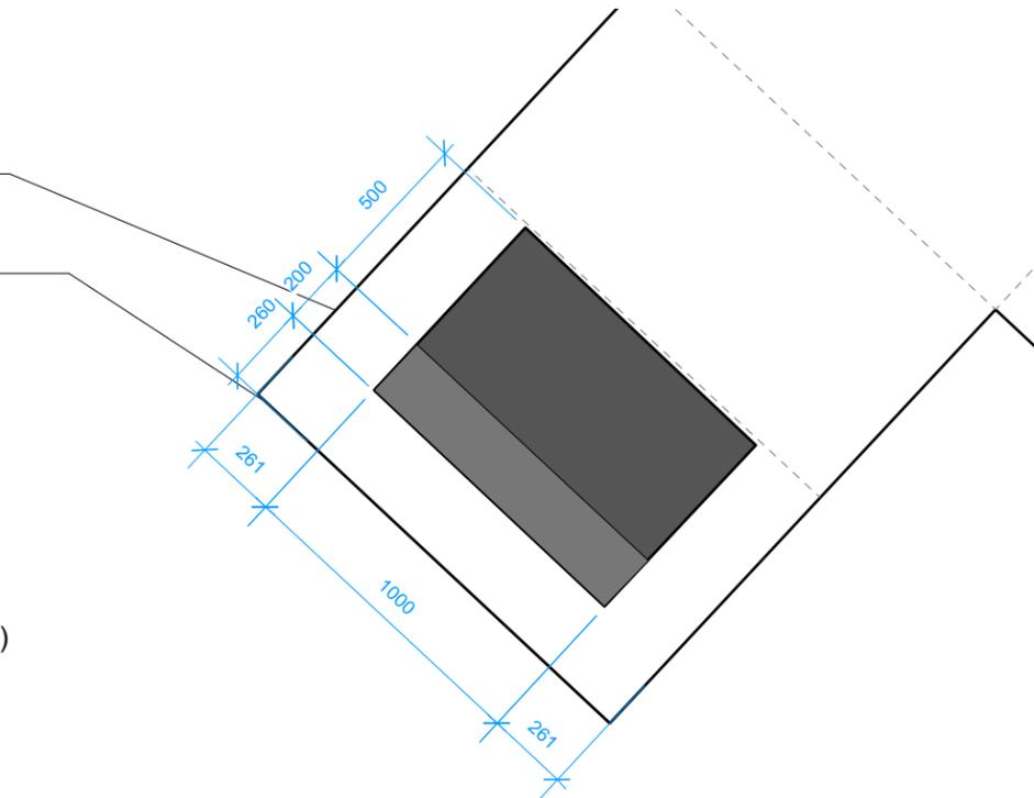
3 PLINTH ON THICKENED CONCRETE PAD (PLAN)
